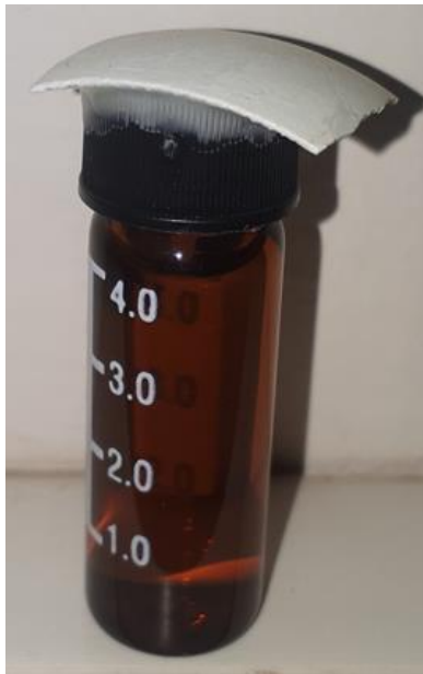
Figure 2.6: View of a test unit with an African Penguin eggshell fragment glued onto the vial cap.
