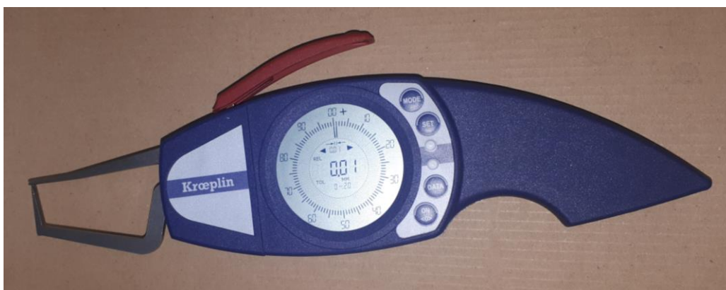
Figure 2.4: The digital calliper (Kroeplin B2R20S) that was used to measure eggshell thickness.
