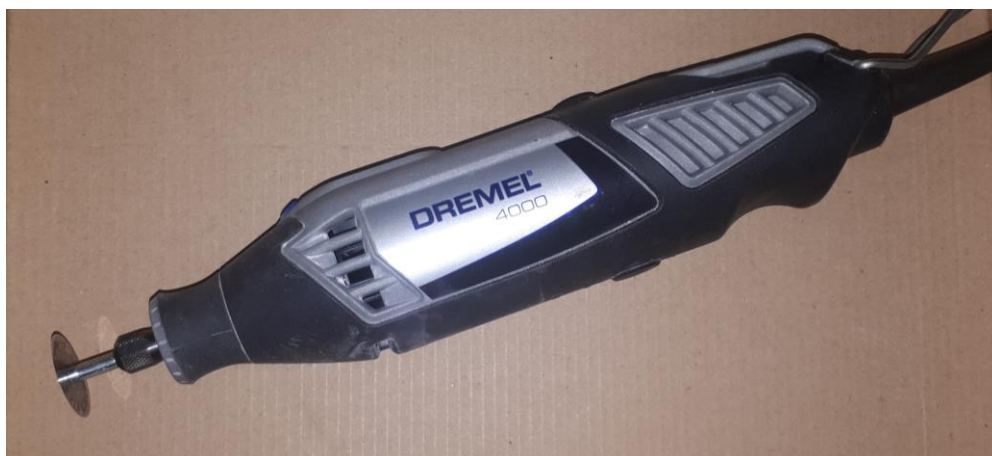
Figure 2.3: The Dremel 4000 rotary tool with a 25 mm steel Mini Blade wheel that was used to cut the eggshells into square fragments.
