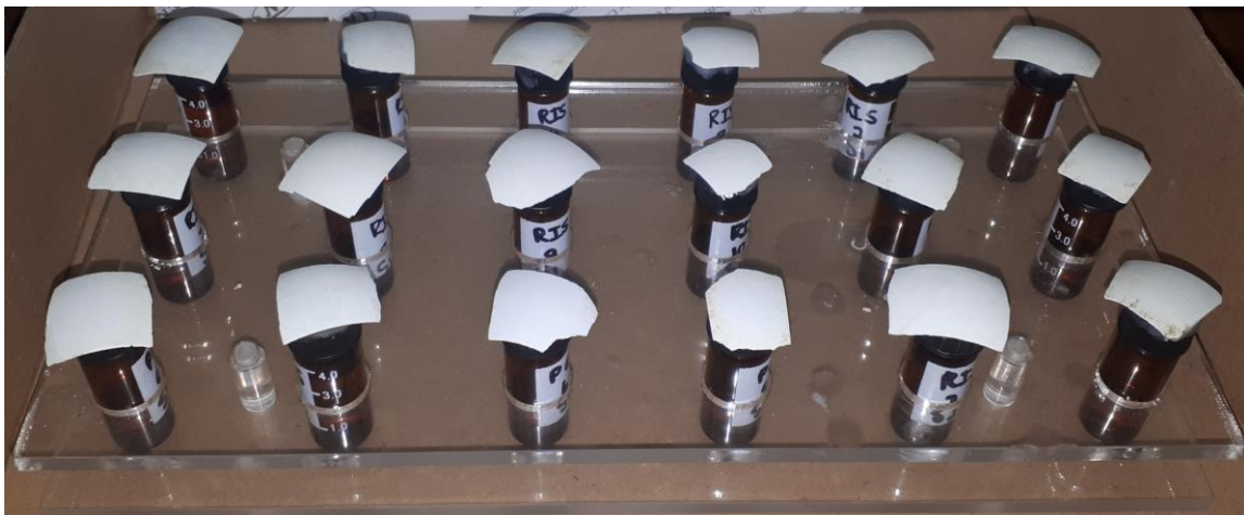
Figure 2.7: Tray holding eggshell test units for treatments.
