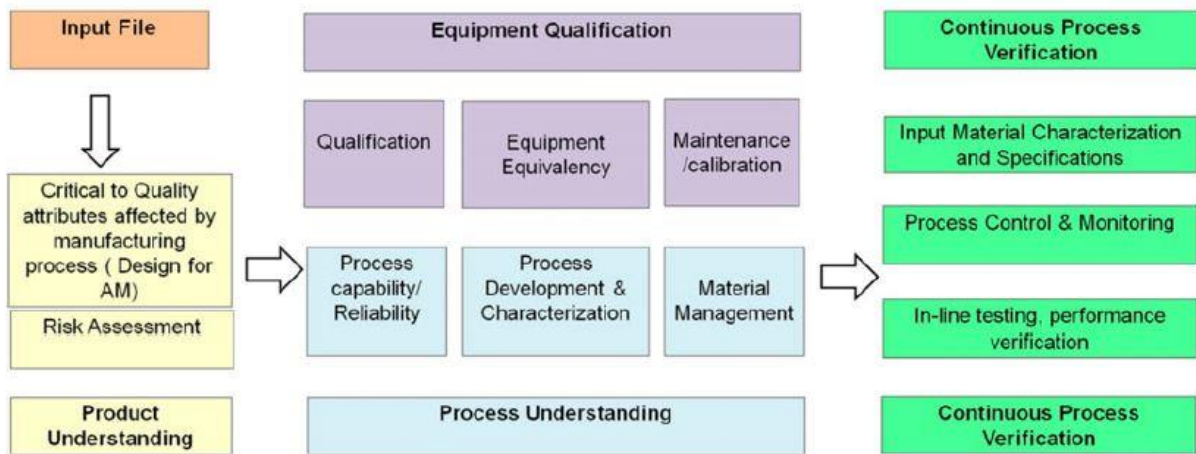
Figure 3 4: A Quality Management Framework for Additive Manufacturing for Medical Devices
