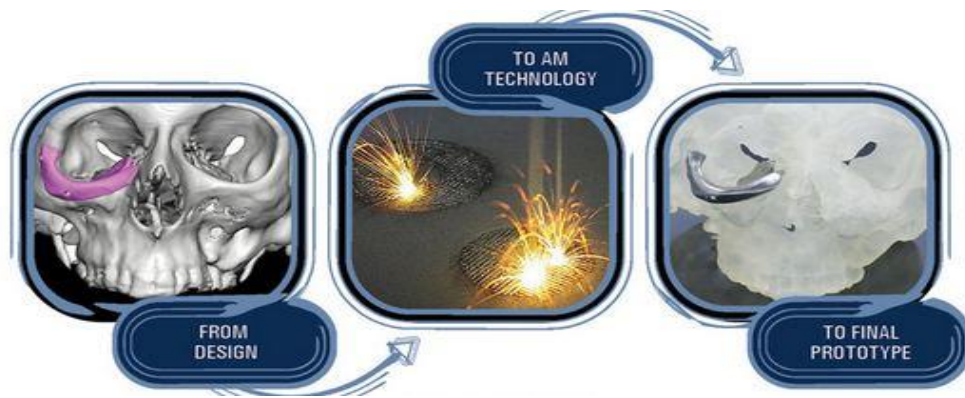
Figure 1. 6: Process of Creating Prosthesis for Medical Implant, from Design to Final Prototype at CRPM. Source: CRPM website ( http://www.cut.ac.za/crpm/ )
