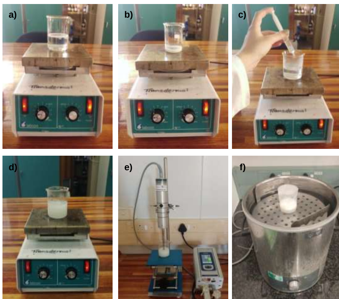
Figure C.1: Formulation method of the (NE1) : a) water and Tween® 80 preheated (phase B); b) safflower oil, Span® 60 and artemether preheated (phase A); c) phase A was added to phase B by means of a syringe; d) mixing of phases A and B together; e) sonication through 3 min ultrasonic probe and f) dispersion was placed in the ultrasonication bath
