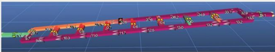
Figure 2. Example coal fire after 30 minutes – showing airflow reversal in parallel airway.
