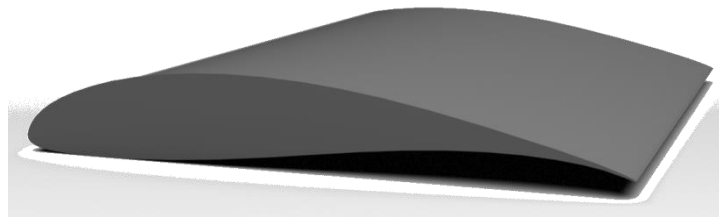
Figure 24: FX 63-137 Aerofoil CAD model for Star-CCM+ simulation
