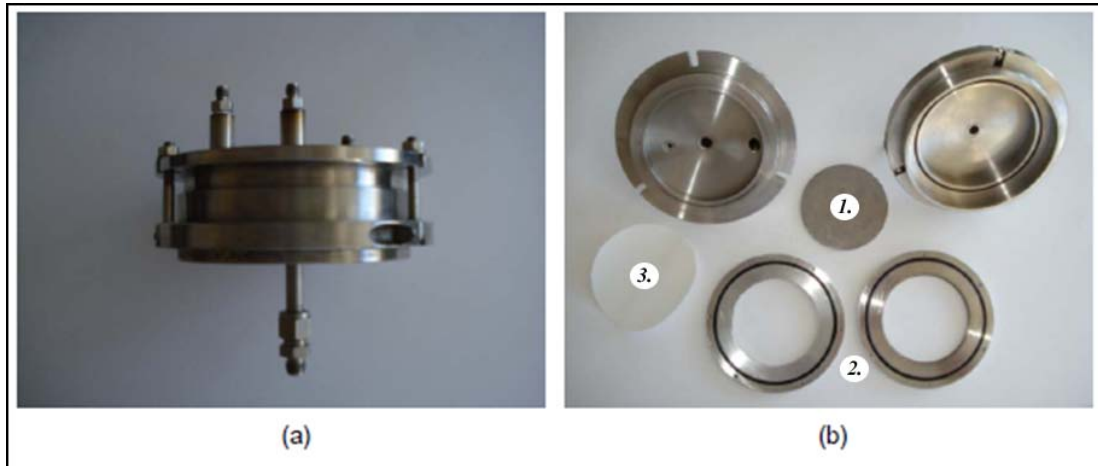
Figure 3-3: Membrane module photo
