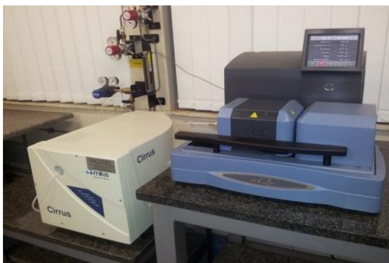
Figure 3.7: SDTQ 600 TGA coupled to MKS quadrupole MS
