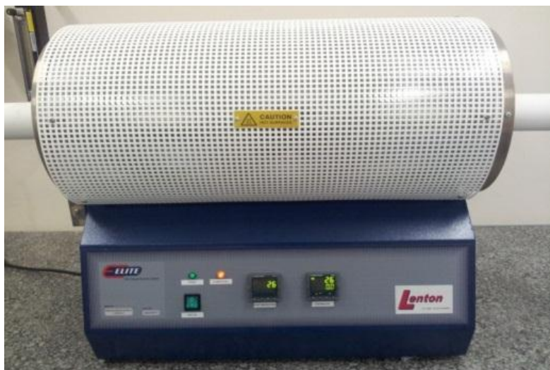
Figure 3.8: The tube furnace used to collect larger volumes of products
