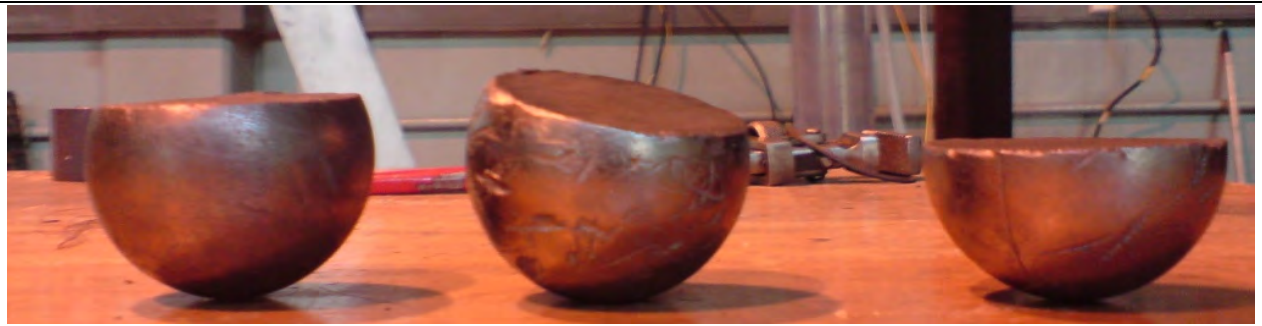
Figure 72: Unusable sphere size range that could cause blockage in lifting line
