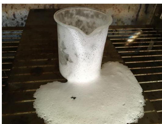
Figure D.1: The outcome using the vacuum oven for degassing the gel
