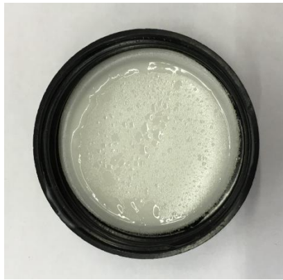
Figure F.6: Signs of condensation on the inside of the lids of the cream containers
