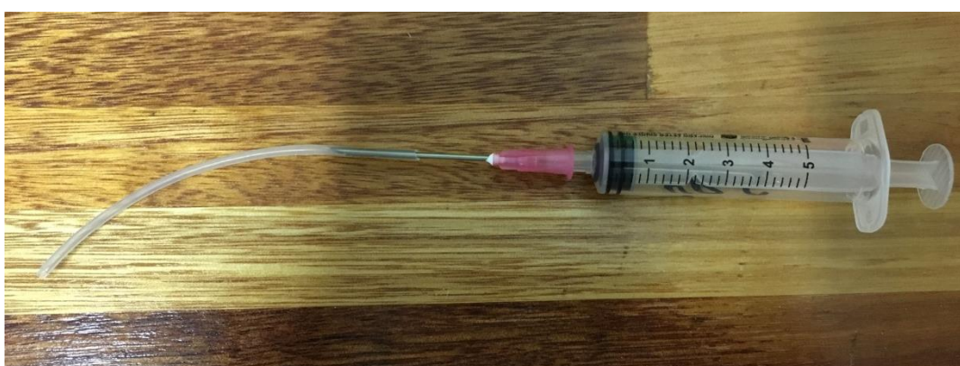
Figure G.5: Syringe (5 ml) and 18 gauge needle with silicon tube used to extract and replace the receptor compartment
