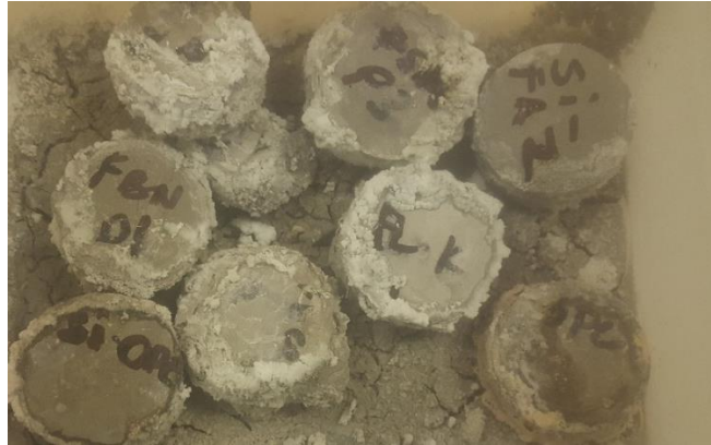
Figure 4.3: The formation of white crystals on unconditioned \text{Ca}(\text{OH})_2 activated fly ash type geopolymers.
