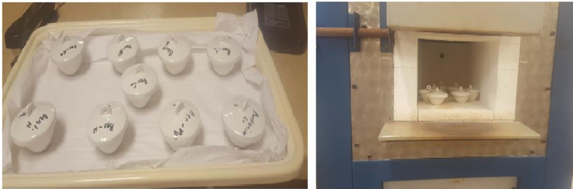
Figure 4.1: Candidate mineral clays placed in a furnace at 700°C for 3 hours.
