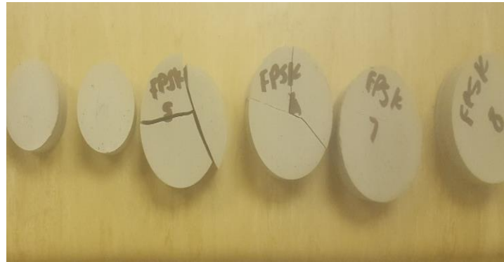
Figure 4.2: Cracking of KOH activated geopolymers during ambient unsealed curing.
