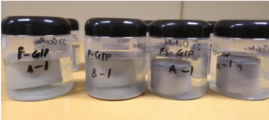
Figure 4.10: A visual illustration of fly ash (F-GIP) and fly ash/silica fume (FS-GIP) geopolymers immersed in 10% sulphuric acid solution after 2 days of exposure.
