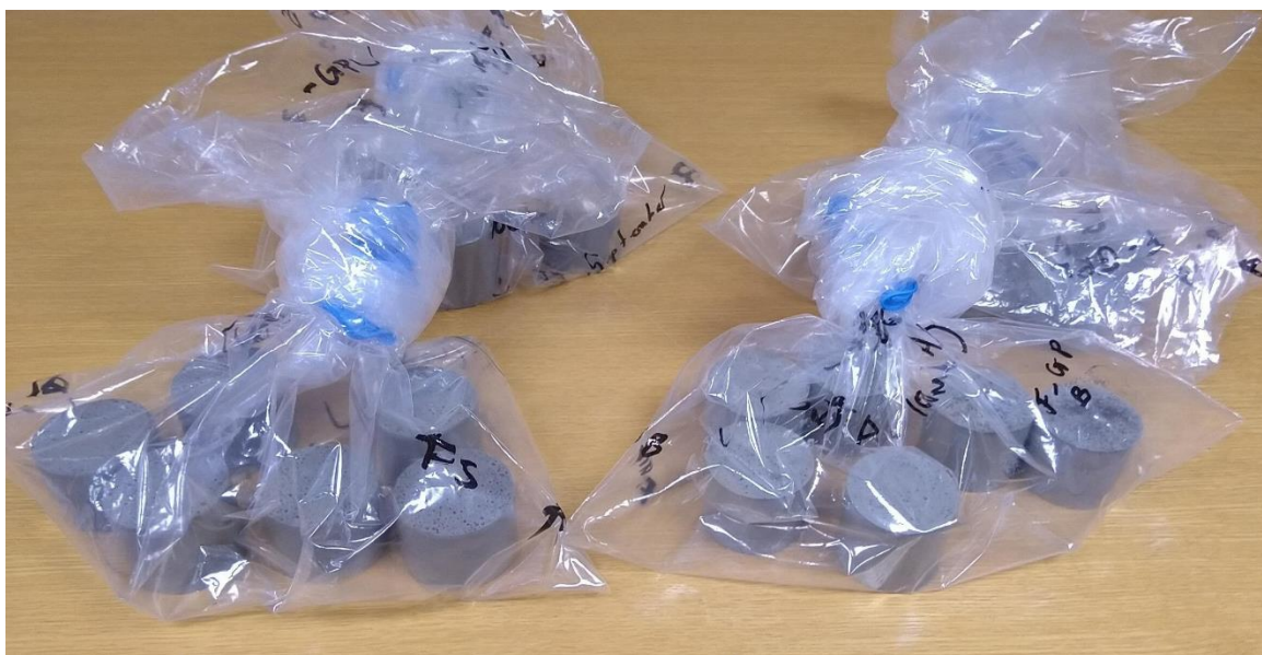
Figure 4.4: Geopolymer candidate samples cured in sealed plastic bags.
