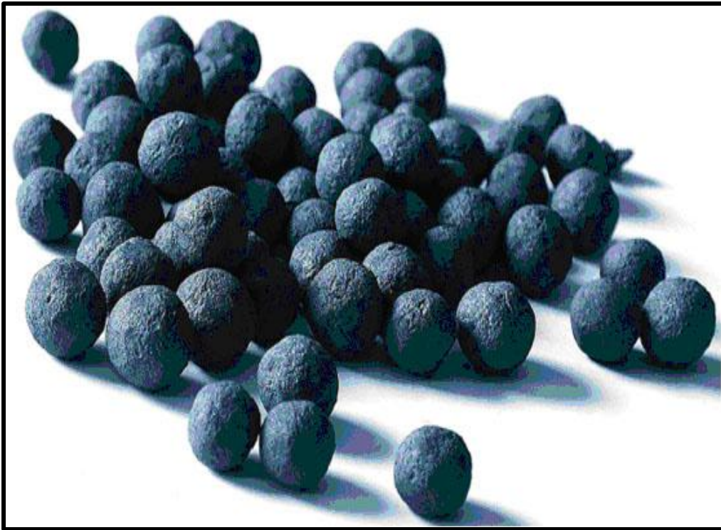
Figure B-4: Typical industrially prepared chromite ore pellets
