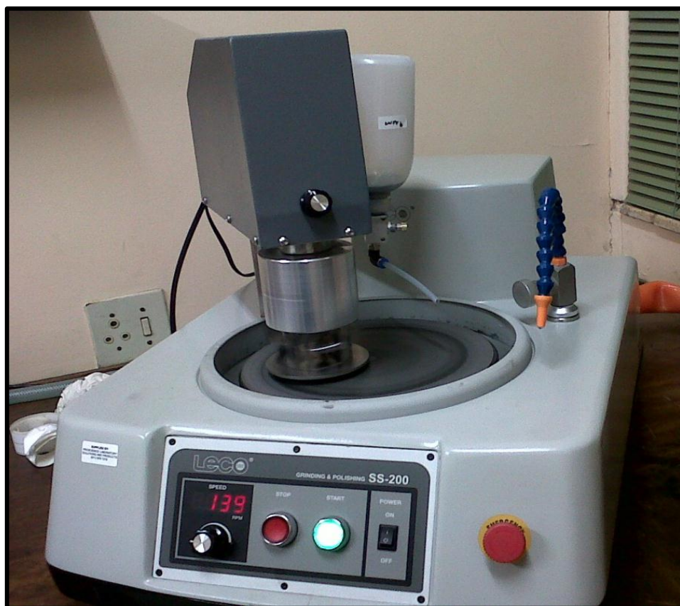
Figure 3- 2: An image of a SS20 Spectrum System Grinder polisher, polishing three moulded chromite pre-reduced pellets at the same time with diamond paste suspension dripping at a set flow rate while the disc rotates at 139 rpm
