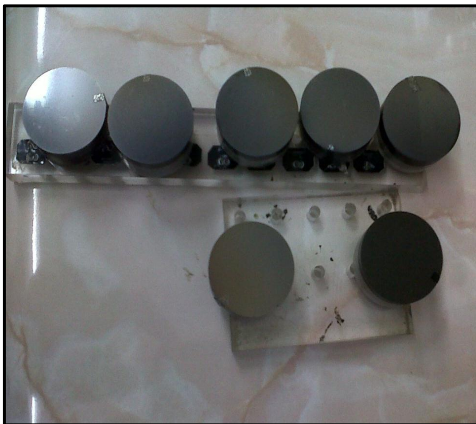
Figure 3- 4: Typical moulded, polished and carbon-coated samples of pre-reduced pellet mixtures
