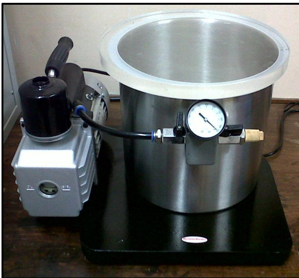
Figure 3- 1: A Speedivac vacuum degassing chamber model VDC 12
