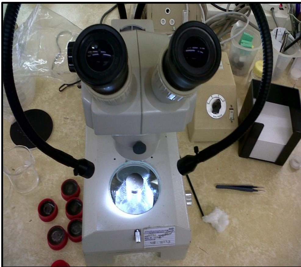
Figure 3- 3: Inspection of sample scratches using a Nikon stereo-spectroscopy
