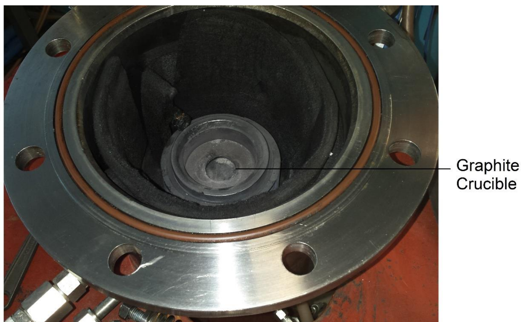
Figure 5-3: The internal structure of the bottom of the plasma reactor
