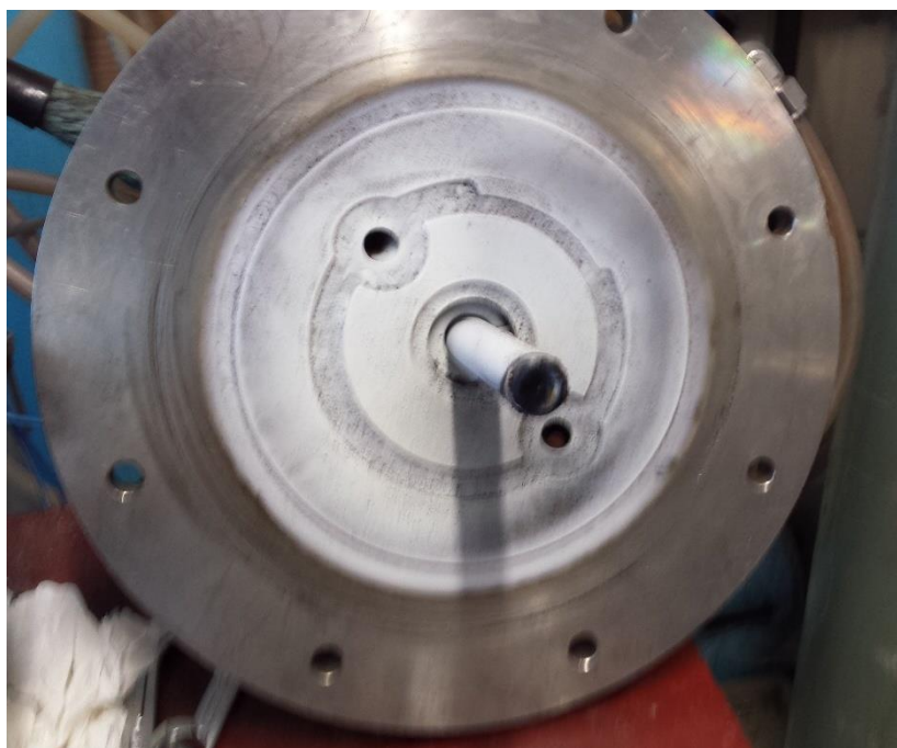
Figure 5-12: Plasma reactor lid with the dispersed white powder
