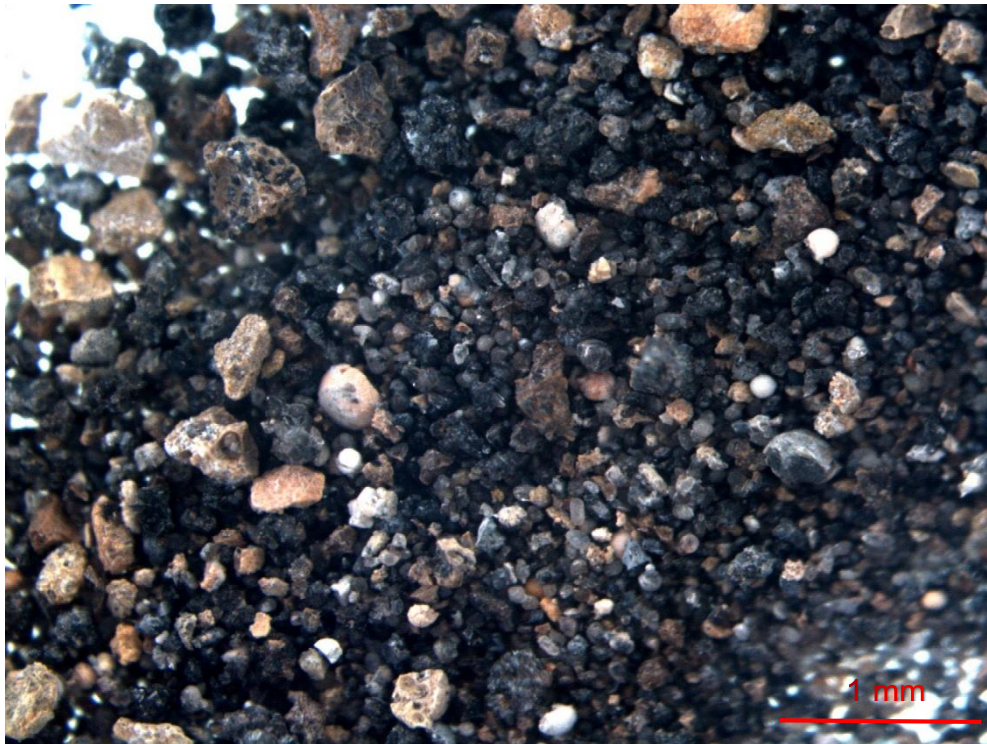
Figure 5-17: Microscopic image of PTM H residue post leaching with 32 % HCl at 80 °C for 1 h
