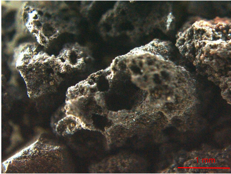
Figure 5-10: Microscopic image of PTM which has been treated in the plasma for too long and melted
