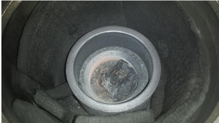
Figure 5-8: Plasma Treated Monazite (PTM) within the graphite crucible after a successful plasma run
