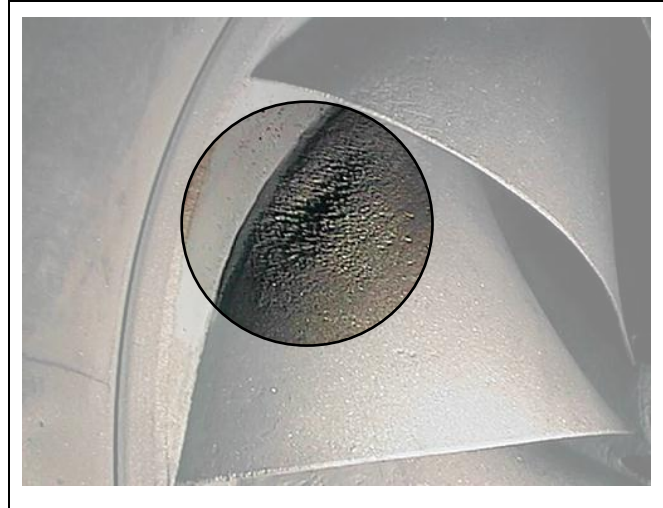
Figure 19: Cavitation pitting on an impeller 7
