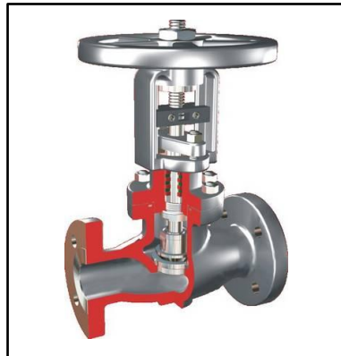
Figure 15: Sectional view of a globe valve 3
