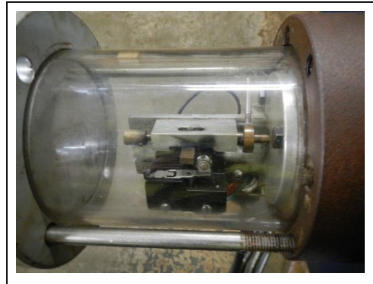
Figure B-4: Pump impeller displacement switch
