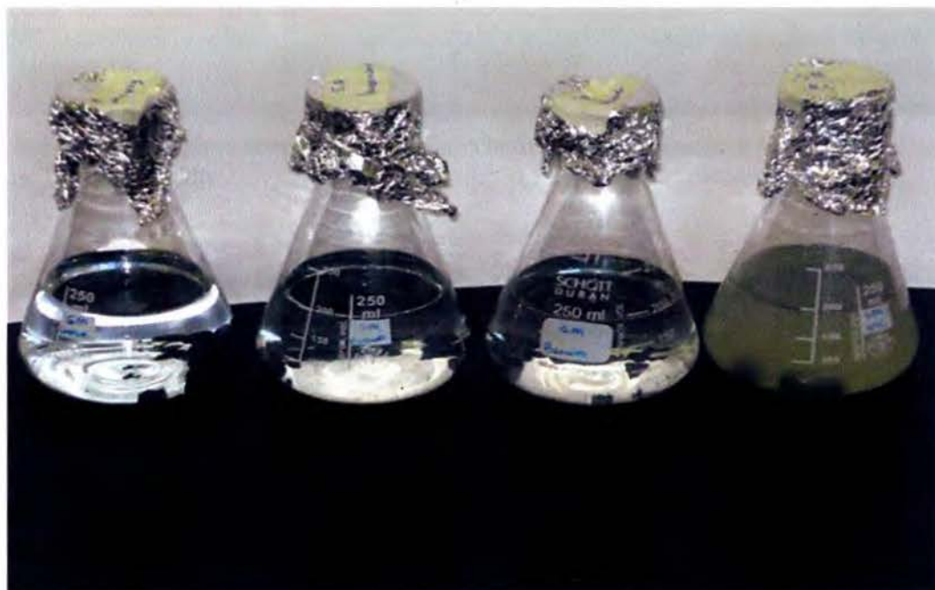
Figure 4.8: Bioreactors containing a graphite chunk and liquid medium without glucose. From Left 1) graphite only; 2) Bacillus subtilis ; 3) Pseudomonas putida ; 4) mixed culture.
