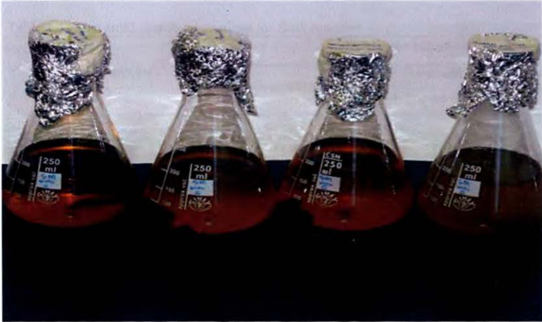
Figure 4.9: Bioreactors containing a graphite chunk and liquid medium with glucose. From Left 1) Graphite only; 2) Bacillus subtilis ; 3) Pseudomonas putida ; 4) Mixed culture.
