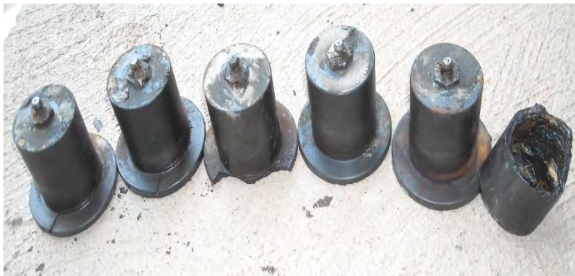
Figure 27: Damaged bushes of IGV
