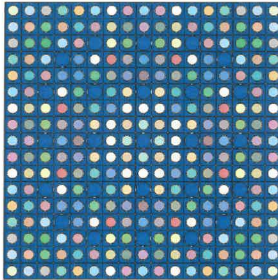
Figure 5-4: Power profile for the standard fuel assembly
