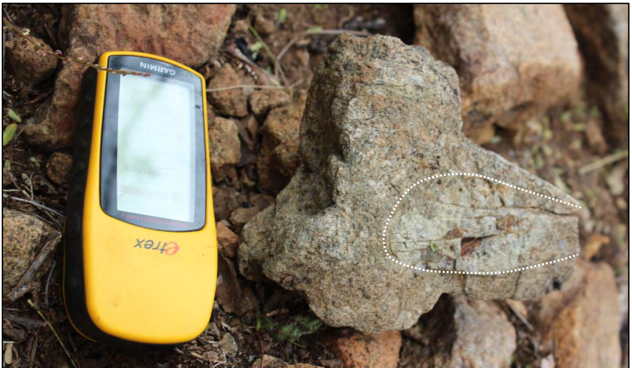
Figure 25: An alkali syenite rock sample containing fine-grained fractured pseudotachylite, found along the upper base contact of the alkali syenite sill.
