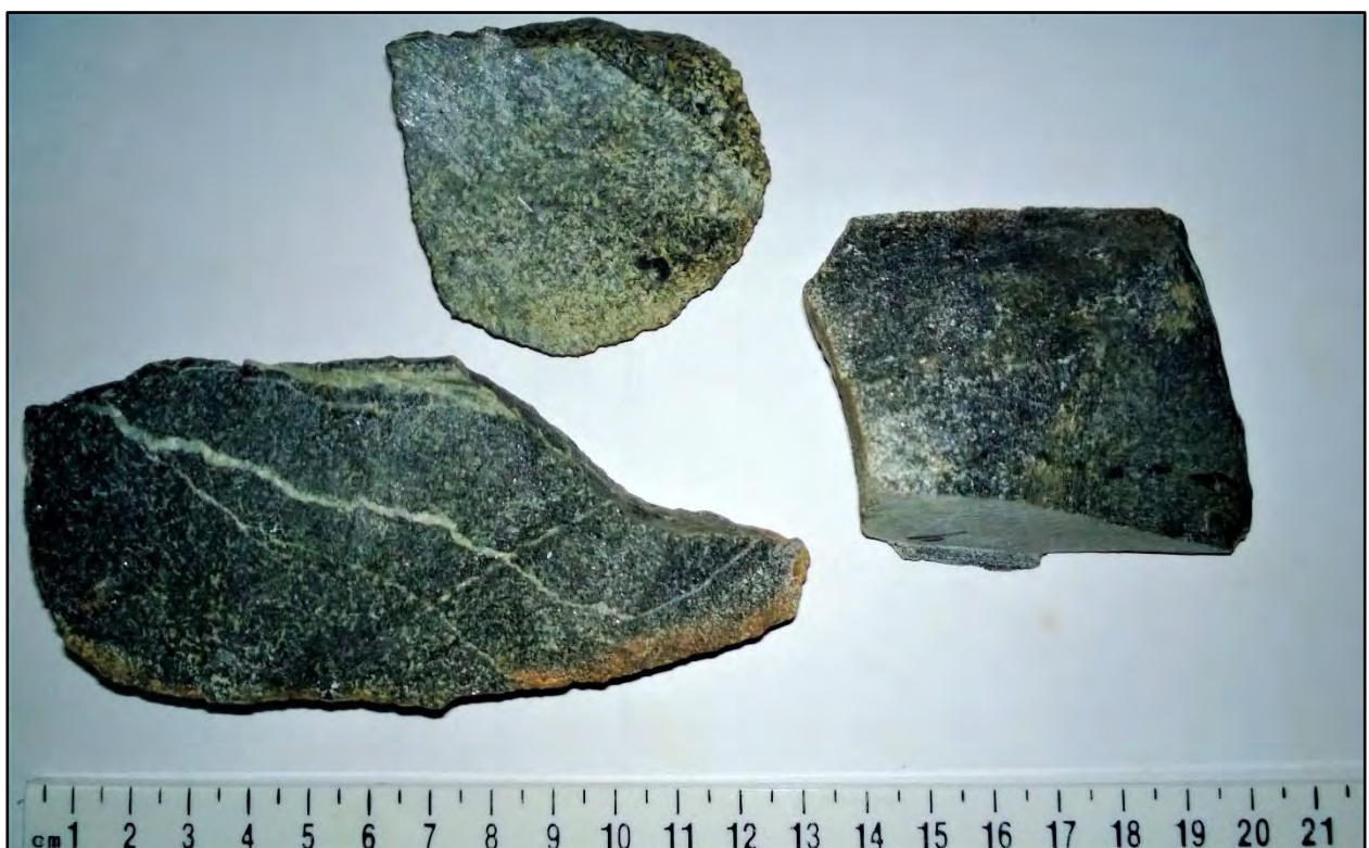
Figure 18: Typical medium-grained gabbroic specimens, from west of fault zone F_2 bordering the northern wehrlite outcrop.
