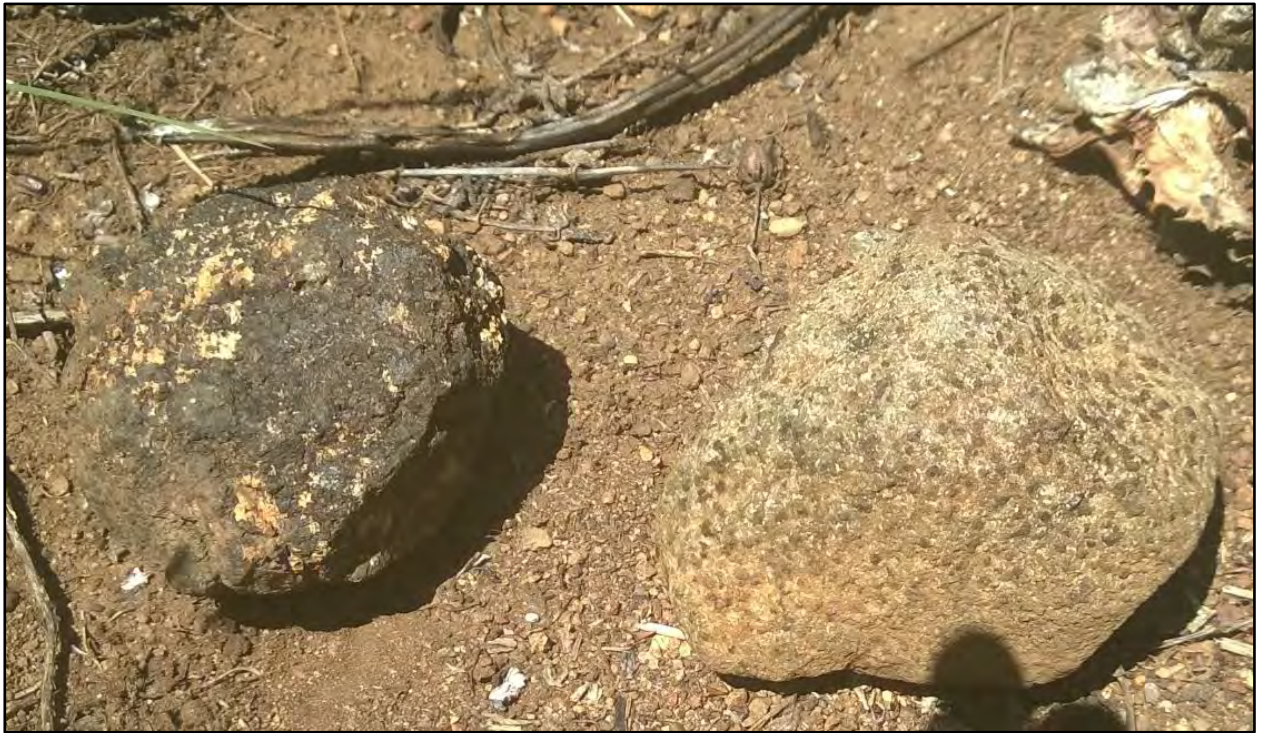
Figure 19: Samples of the melanocratic, equigranular (left) and porphyritic (right) rock types found along the southern portion of the main spessartite body.
