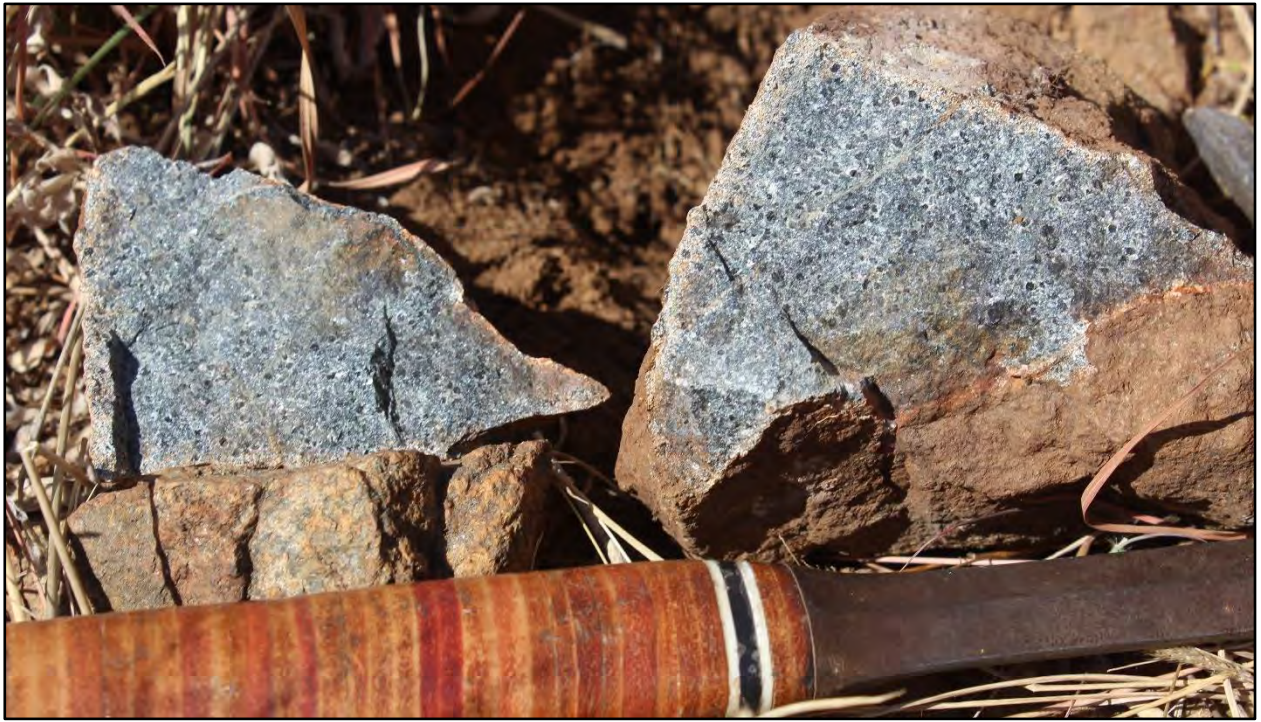
Figure 21: Leucocratic spessartite displaying a poikilitic texture, found along the northern portion of the main spessartite body.
