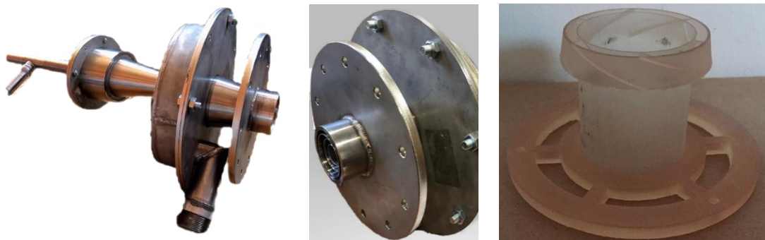
FIGURE 4.41: IMAGES OF: PC BURNER (LEFT AND MIDDLE), SWIRLER CONSTRUCTED FROM HIGH TEMPERATURE RESIN (RIGHT)
