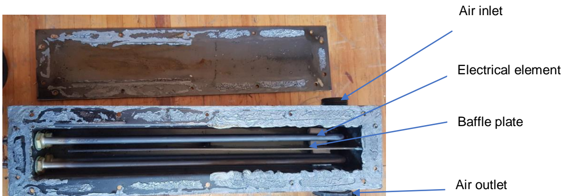
FIGURE 5.6: IMAGE SHOWING INTERNAL VIEW OF ACTUAL CA HEATER
