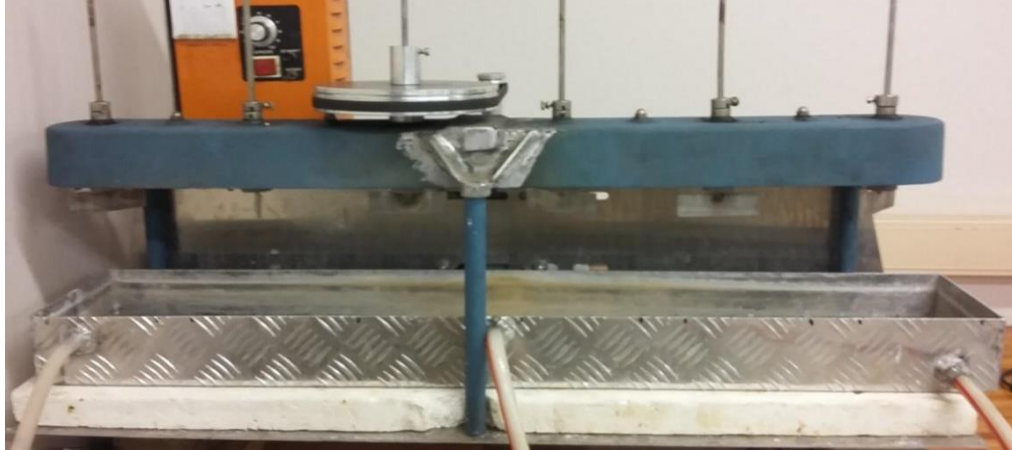
Figure 4-1: Jar test apparatus with a tray
