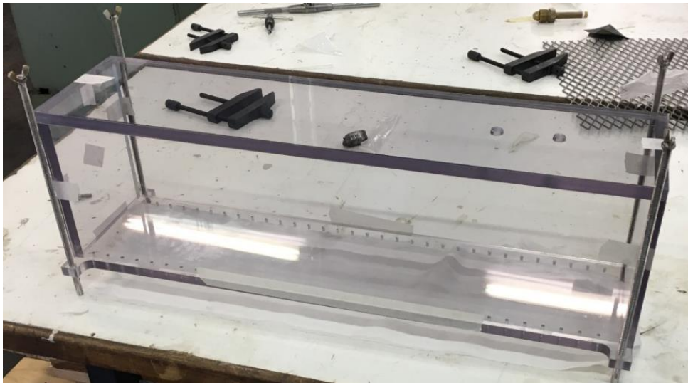
Figure 3-8: Drip tray prior to installation inside evaporation chamber
