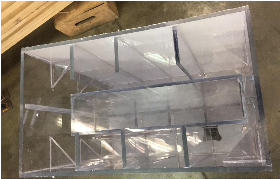
Figure 3-12: Gluing of polycarbonate to form evaporation chamber.
