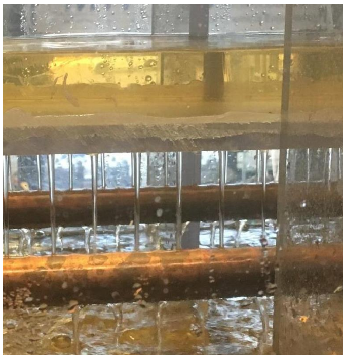
Figure 3-21: Drip tray's laminar water flow distribution onto heat exchange surfaces
