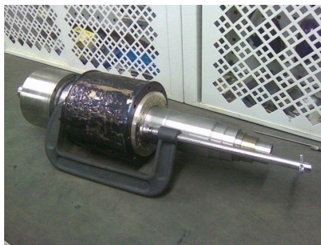
Figure 4-14: Inserting the 3mm dowel pins into the bars
