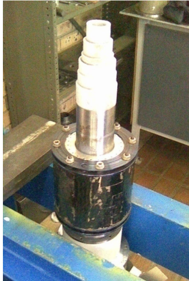
Figure 4-13: Picture of the assembled IM rotor section onto the shaft
