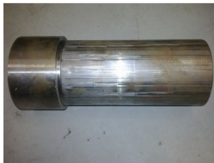
Figure 4-10: Illustration of the jagged mandrel surface due to the bottom spacer removing material
