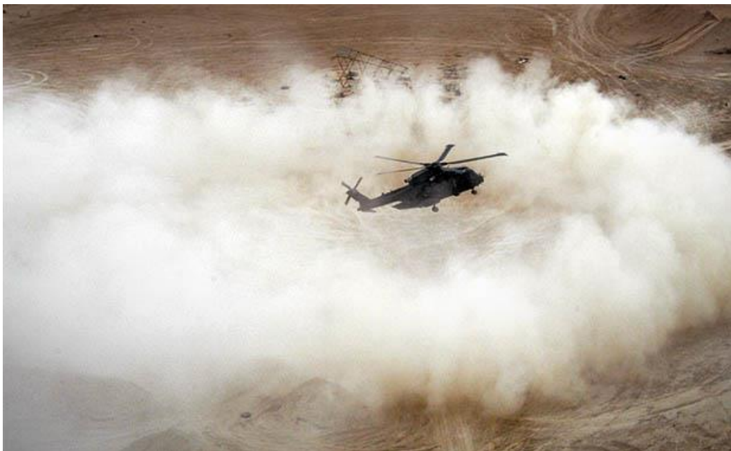
Figure 97. Brownout generated by EH-101 during IGE hover flight [LZDZ, 2017]
