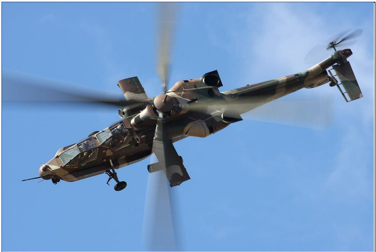
Figure 78. The main downwash-inducing agents: Main Rotor Hub, Blades, Engines and Fuselage [Gary Shephard, 2008]
