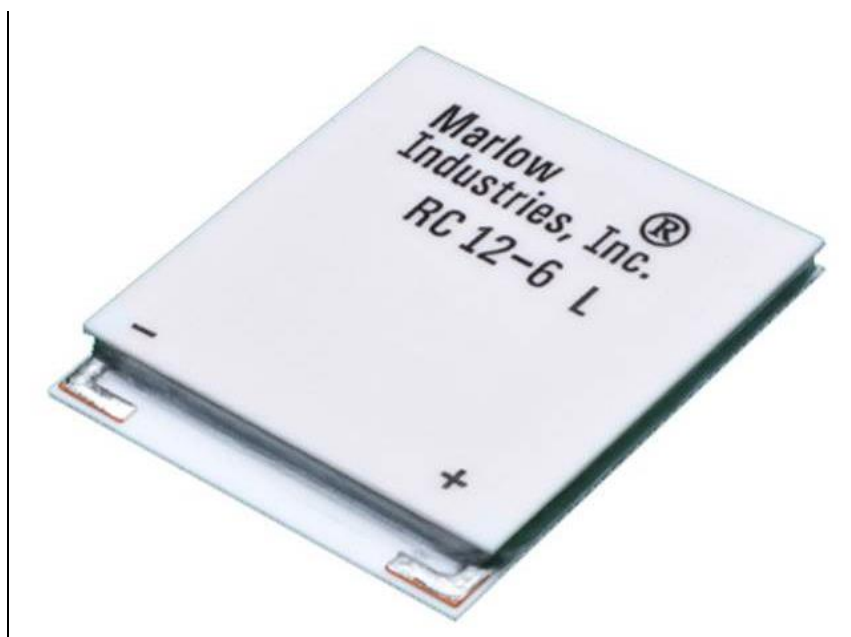
Figure 148. Physical outline of MARLOW Peltier device RC12-6L [MARLOW, 2018]
