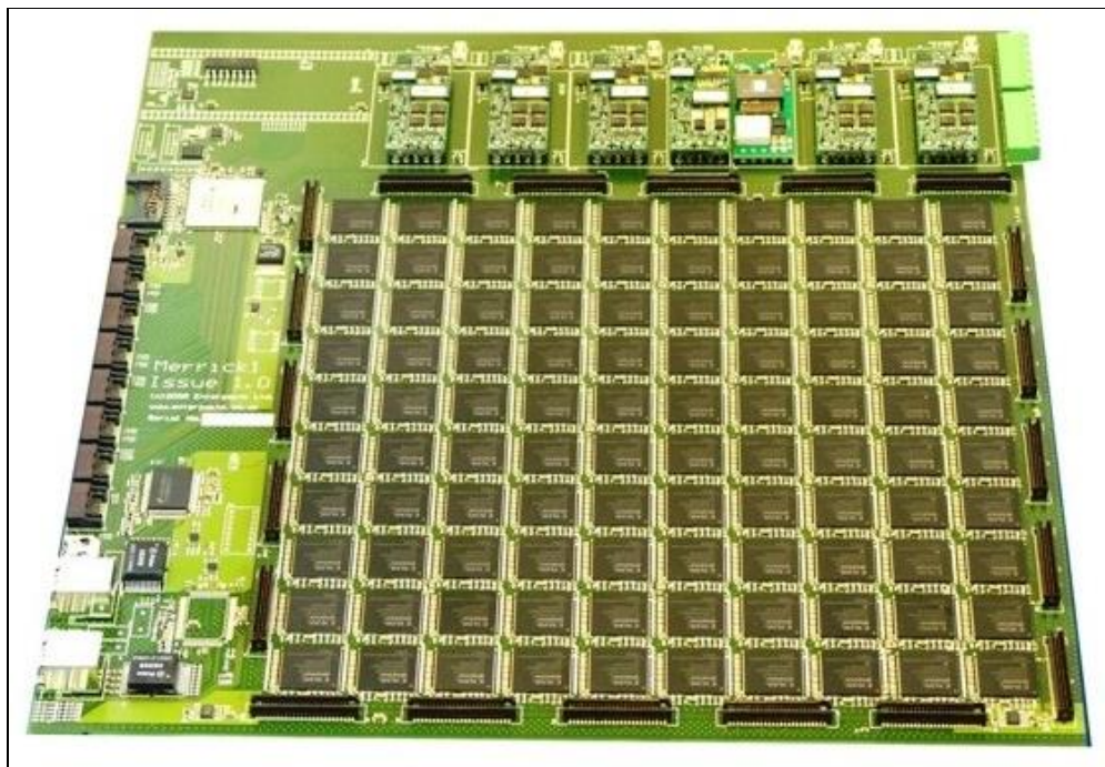
Figure 150. Merrick1 board with 10x10 SPARTAN FPGA Array [Enterpoint, 2016]
