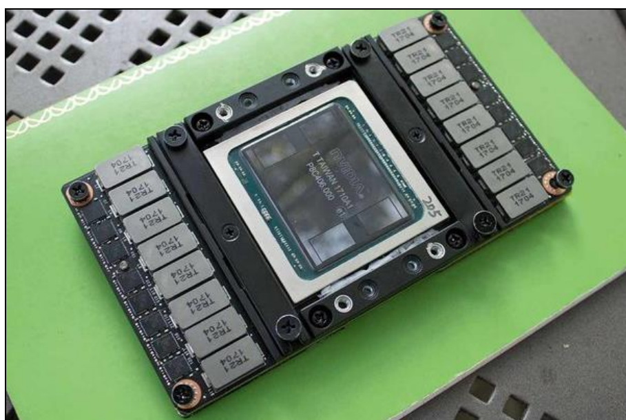
Figure 130. NVIDIA TESLA V100 card with P8C406000 GPU, top view [Paul Alcorn, 2017]
