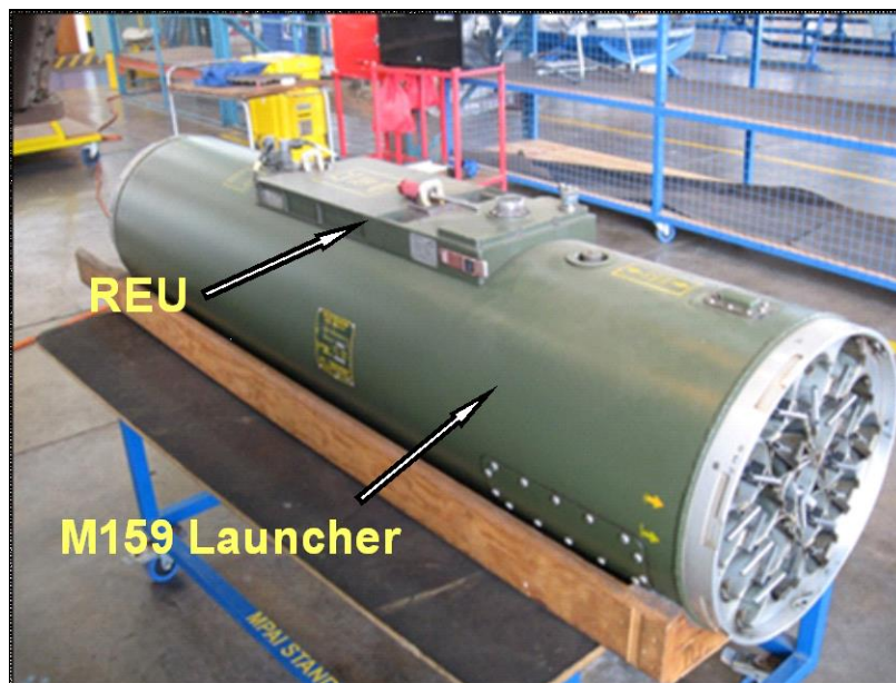
Figure 121. M159 Rocket Launcher with REU fitted on Rooivalk AH-2A [A Landman, 2014]
