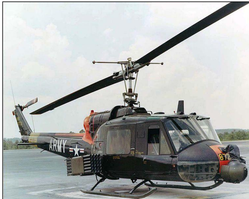
Figure 1. Early weapon system additions to the Bell UH-1 [U.S. Army, 1964]
