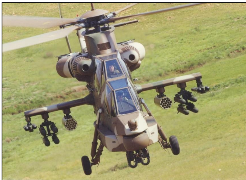
Figure 3. Rooivalk AH-2A with typical weapons config [Denel Aeronautics, 2010]
