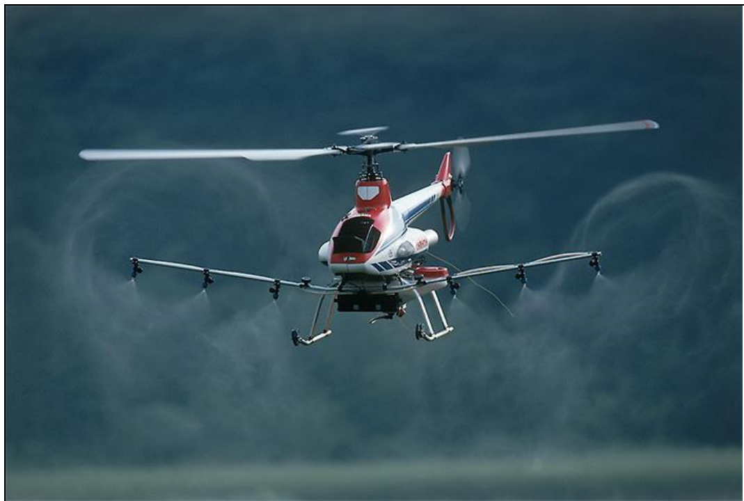
Figure 99. Downwash of R-50 morphing into two downward tail at rear [Yamaha, 1987]
