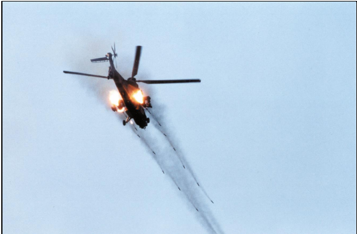
Figure 13. Skewing rocket trajectories during qualification of RLS on Rooivalk AH-2A [Wes Lindenberg, 2013]
