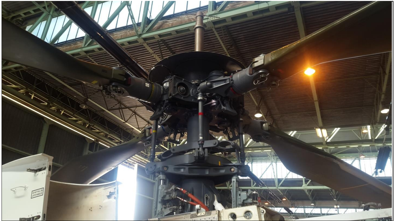
Figure 79. The Main Rotor of Rooivalk AH-2A [A Landman, 2018]
