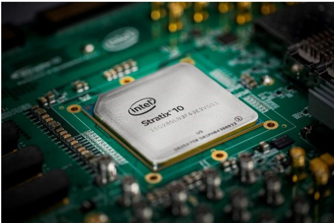
Figure 168. Exterior view of Stratix 10 BGA package [Intel: 2016]
