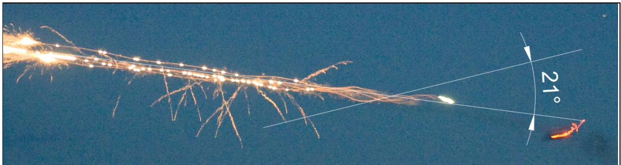
Figure 18. Estimating Coning Angle [A Landman, 2017]
