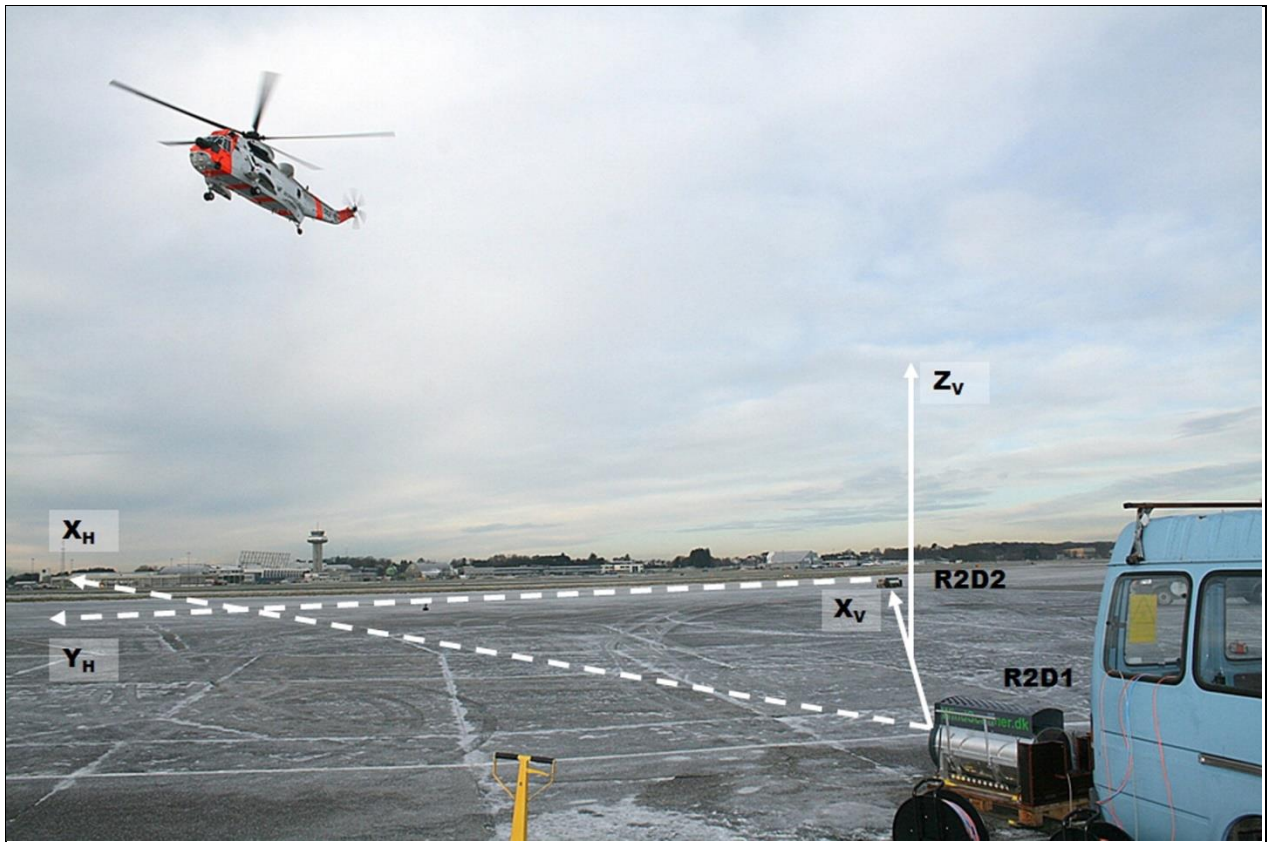
Figure 100. Using two LIDAR's to measure air velocity below SH-3 Sea King helicopter [Sjöholm et al, 2014]
