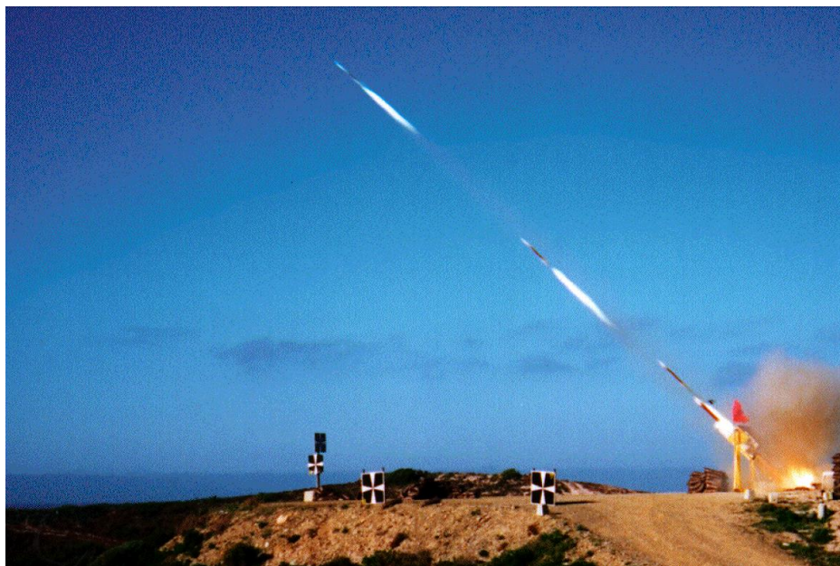
Figure 49. FZ90 Motor with FZ181 Warhead being launched from Ground Jig [Onno Sakkers, 1997]
