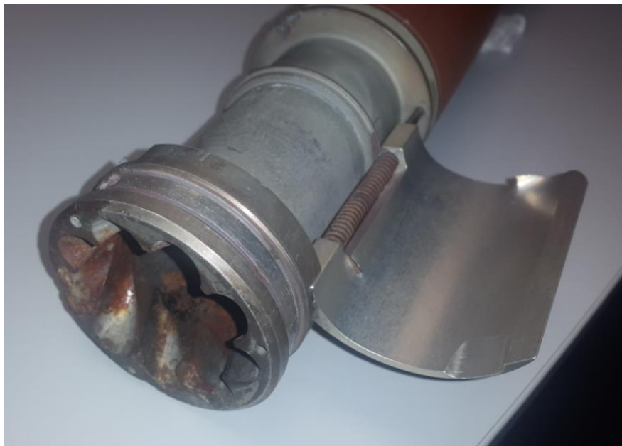
Figure 57. Wrap-Around Fin and Nozzle of a recovered FZ90 Rocket Motor [A Landman, 2017]
