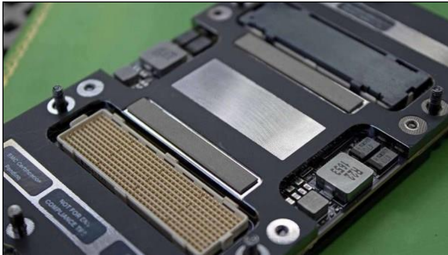
Figure 131. NVIDIA TESLA V100 card with P8C406000 GPU, bottom view [Paul Alcorn, 2017]
