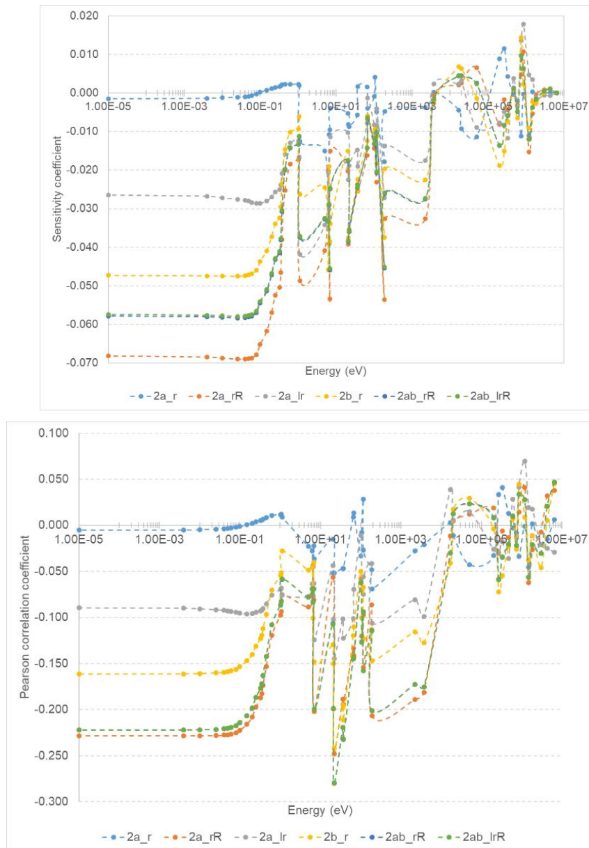
Figure 6-19. ^{238}\text{U}(n,\gamma) / ^{238}\text{U}(n,\gamma) sensitivity coefficients (top) and PCCs (bottom) for various 2a, 2a-2b and 2a-2b-l core models.
