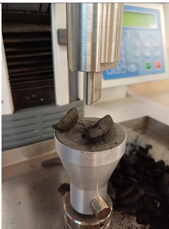
Head used for compressive strength testing
