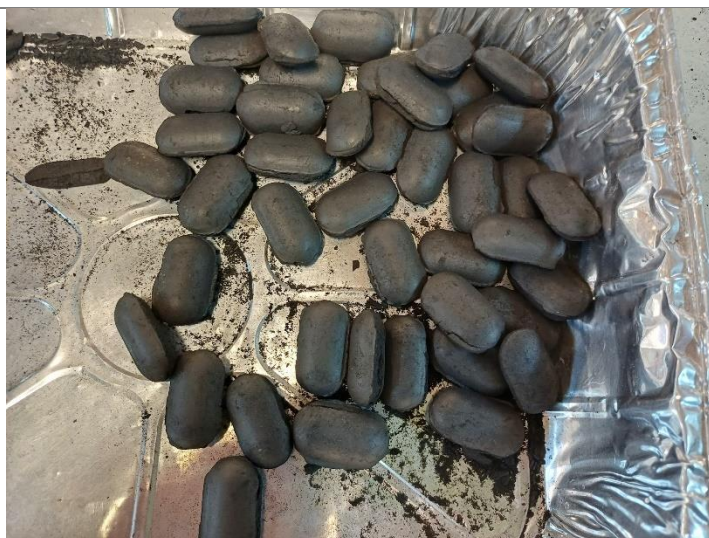
Briquettes produced using biochar (Size of 3.3×1.9×1.2 cm)
