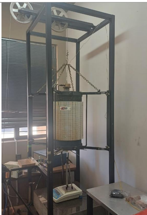
Vertical Elite Thermal Systems Limited tube furnace (Model: TMH16/75/610 3x3216 + 3216i)
