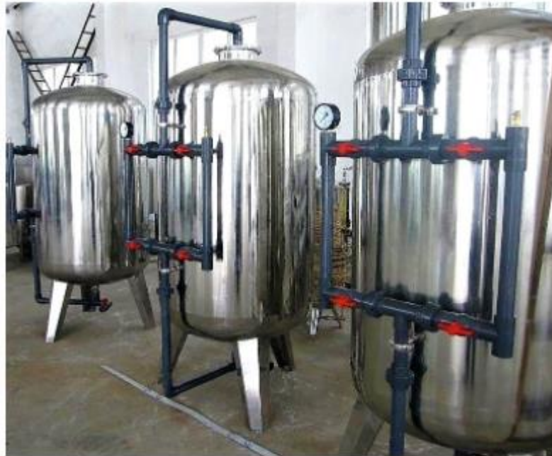
Figure 9: Activated carbon filters (Mazille & Spuhler, 2020b).
