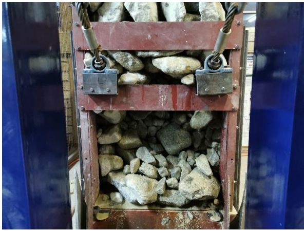
Figure 6-63: Blockage created for the constant load test where the steel cables are used for unblocking a wet interlocking blockage.
