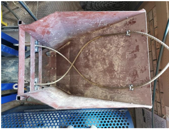
Figure 6-7: Representation of cables laid down in the scaled chute. Left: Top view. Right: Front view.
