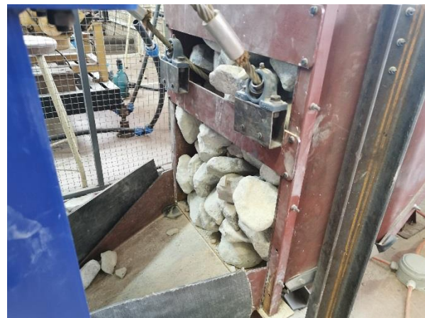
Figure 6-58: Representation of the blockage after 17 consecutive runs for the constant load method with steel cables.
