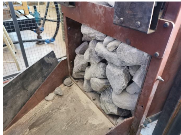
Figure 7-4: Blockage created for the third test frequency where steel cables are caught in a dry interlocking blockage.
