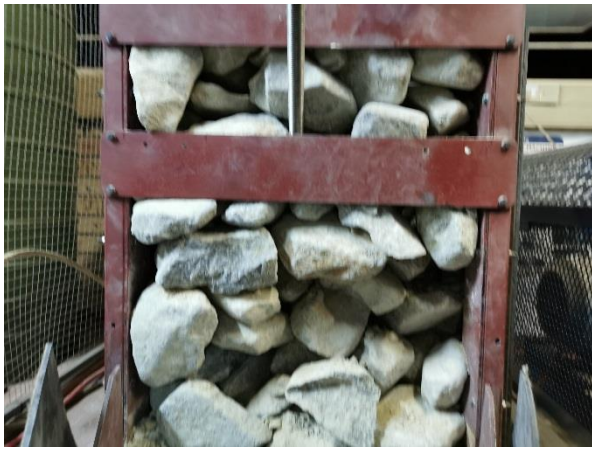
Figure 7-9: Blockage created for the second test where the hammer is for unblocking a dry interlocking blockage.
