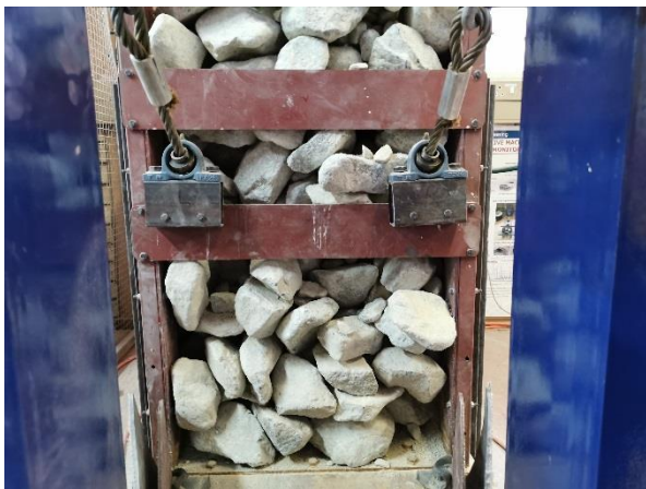
Figure 6-58: Representation of the blockage after 17 consecutive runs for the constant load method with steel cables.
