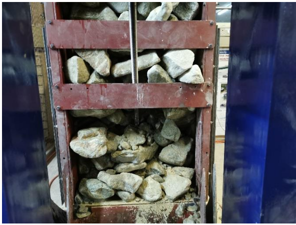
Figure 6-66: Blockage created for the constant load test where the hammer is used for unblocking a wet interlocking blockage.
