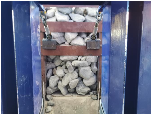
Figure 7-4: Blockage created for the third test frequency where steel cables are caught in a dry interlocking blockage.
