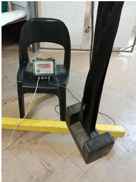
Figure 5-2: Representation of weights weighed to determine the accuracy of the load cell.
