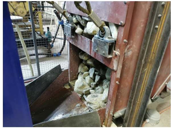
Figure 6-63: Blockage created for the constant load test where the steel cables are used for unblocking a wet interlocking blockage.
