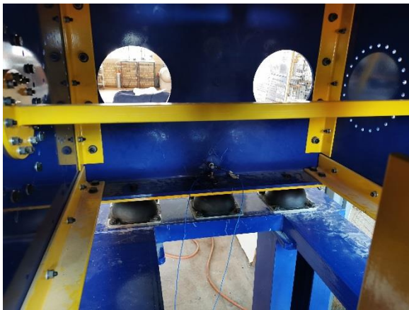
Figure 6-2: Placement of the accelerometers on the machine.
