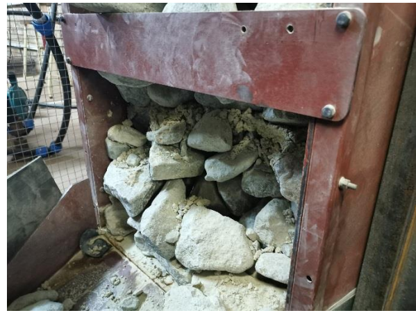
Figure 6-45: Blockage created for the first hammer test with the gate of the chute removed.
