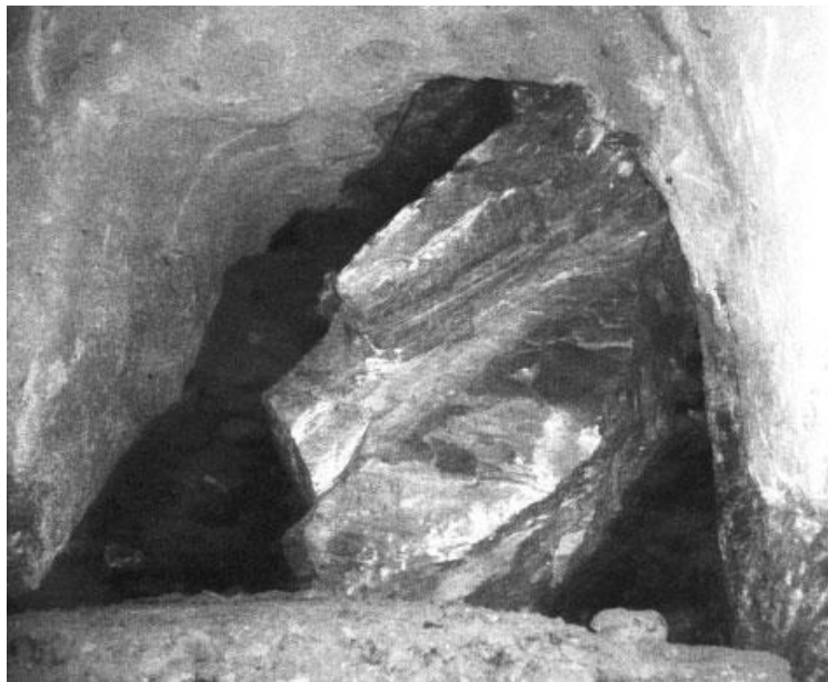
Figure 1-2: A photo of a large rock blocking an ore pass and causing a restriction to the flow of ore and waste rock (Szwedzicki, 2007).
