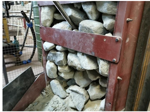
Figure 7-9: Blockage created for the second test where the hammer is for unblocking a dry interlocking blockage.
