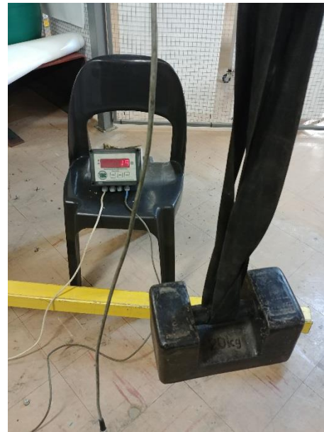
Figure 5-2: Representation of weights weighed to determine the accuracy of the load cell.
