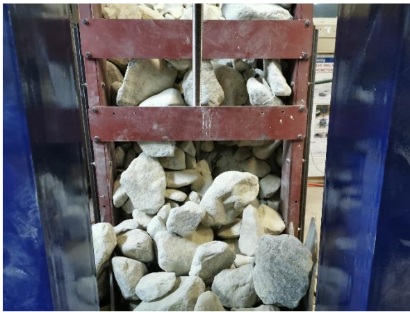
Figure 6-61: Representation of a successful unblocking of the blockage by utilizing a constant load method with the hammer operation.
