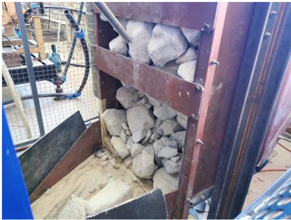
Figure 7-12: Small partial unblocking for the second test where the hammer is used for unblocking a cemented blockage at an excitation unbalance of 50 %.
