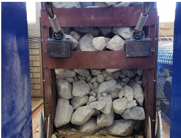
Figure 7-8: Partial unblocking for the second test, at 77 % excitation unbalance, where steel cables are used for unblocking a cemented blockage.
