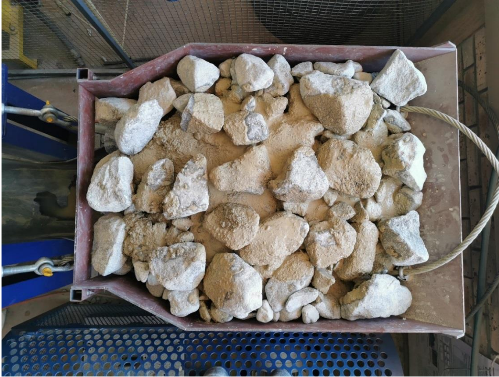
Figure 6-35: Representation of the mud as poured over the sample rocks.
