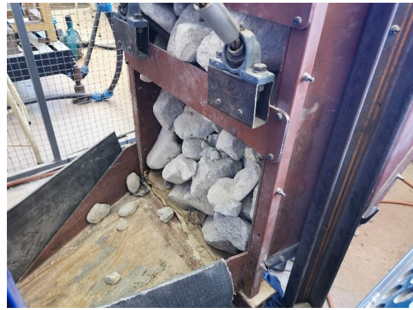
Figure 7-7: Blockage created for the second test where cables are caught in a cemented blockage.
