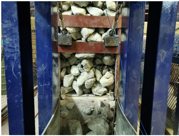
Figure 7-5: Partial unblocking occurred at 20.25 Hz and an unbalance of 94 % for the third test frequency where steel cables are used for unblocking a dry interlocking blockage.
