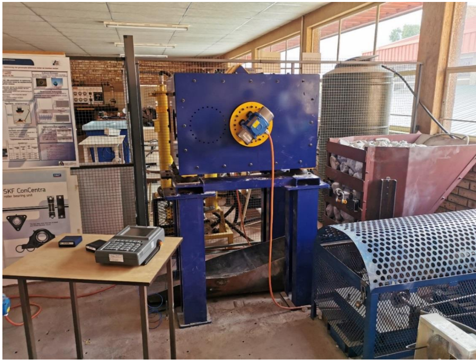
Figure 6-1: Experimental test setup of the machine and chute.
