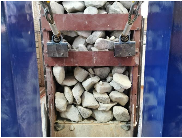
Figure 6-57: Blockage created for the constant load test where the steel cables are used for unblocking a dry interlocking blockage.
