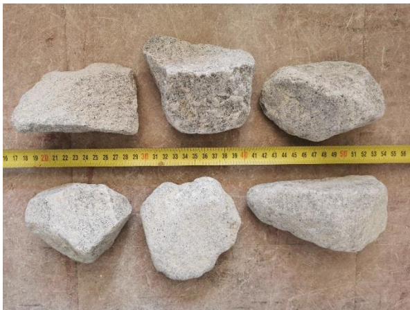
Figure 5-15: Representation of the size of the large medium sample rocks.
