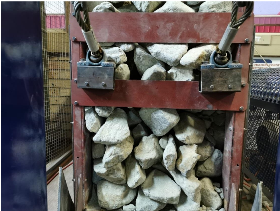
Figure 6-10: Representation of the gate removed from the scaled chute.
