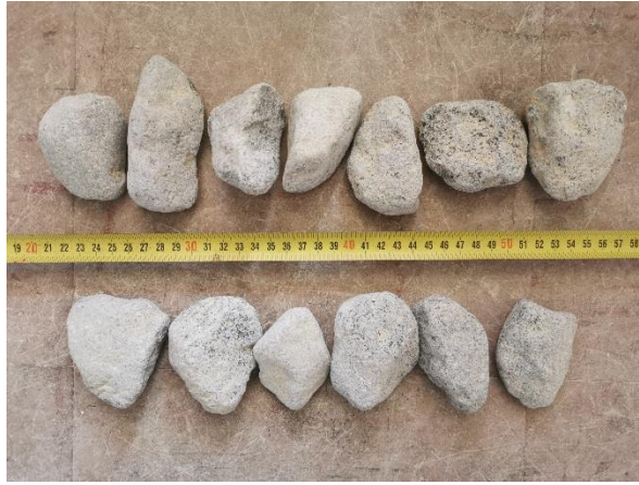
Figure 5-16: Representation of the size of the small medium sample rocks.
