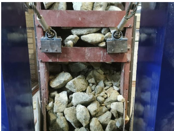
Figure 6-64: Representation of a successful unblocking of the wet interlocking blockage by using a constant load method with the steel cables.
