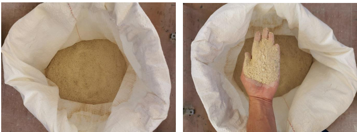
Figure 6-36: Representation of the fine segregated powder with which the mud was created.
