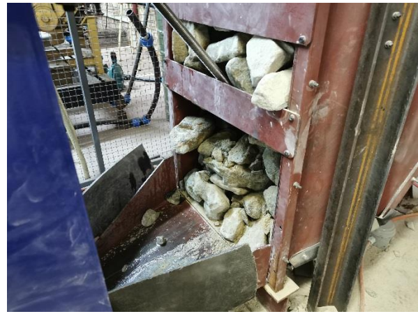
Figure 6-66: Blockage created for the constant load test where the hammer is used for unblocking a wet interlocking blockage.
