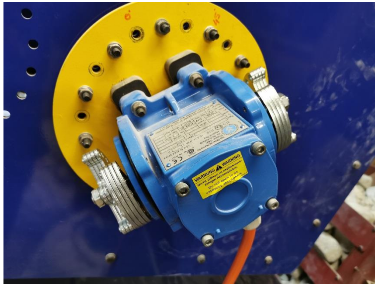
Figure 5-12: One excitation motor of the machine with end caps removed.
