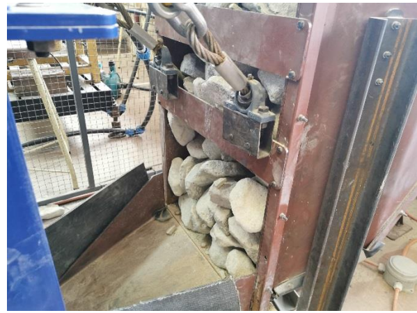
Figure 6-57: Blockage created for the constant load test where the steel cables are used for unblocking a dry interlocking blockage.
