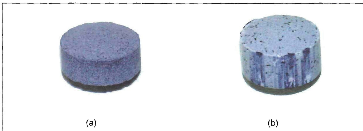
Figure 3.7: Light microscopy of tablet compressed with (a) Avicel ® mixed with 2% w/w magnesium stearate at 69 rpm for 8 minutes and (b) Tablettose ® mixed with 2% w/w Pruv ® at 69 rpm for 8 minutes.
