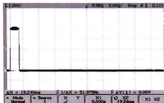
Figure 5.7.1 Control Signal Frequency Measured as 52 Hz
