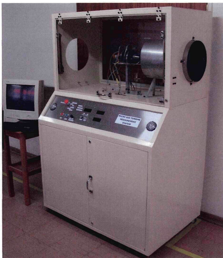
Figure 6.2.1 The Micro Gas Turbine Measurement System
