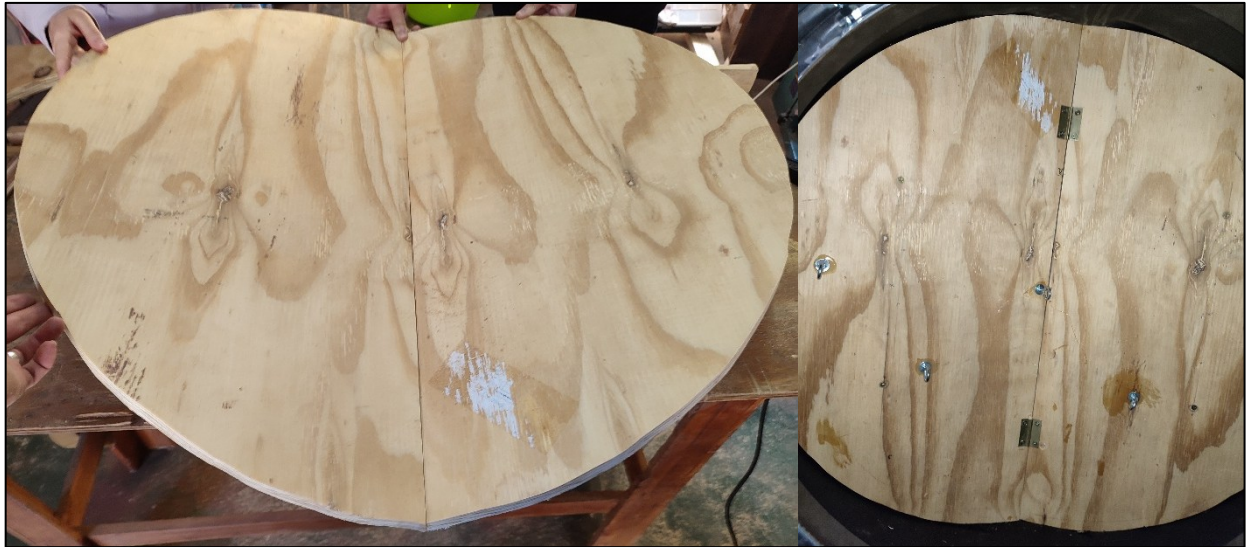
Figure C.2: Inclined wooden base; not assembled (left), and assembled and installed (right)
