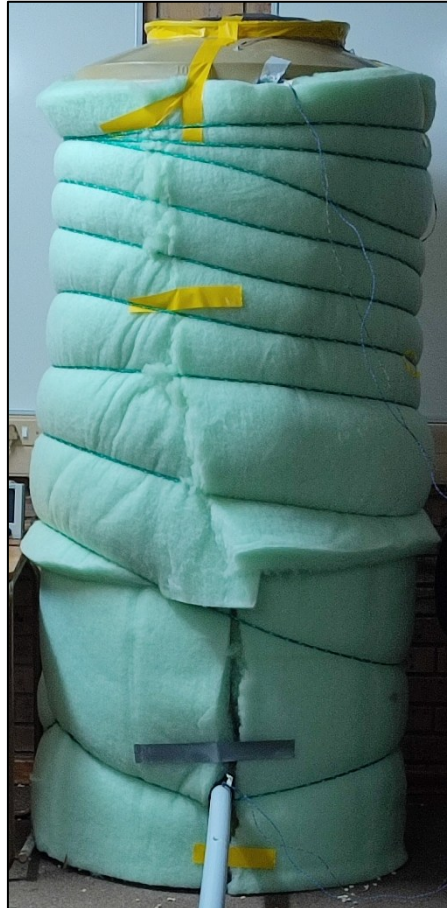
Figure C.1: 1000 litre Slimline JoJo tank wrapped in roofing insulation
