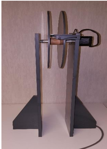
Figure 3-5: Photograph of the rotarod. Mice were placed on the rod as it rotated at 5 rpm. The speed of rotation then increased from 5 to 40 rpm over a period of 5 min. When the animal fell off the rod, the infrared beam above the rod was restored, the rod stopped rotating and the latency to fall (in seconds) was recorded.
