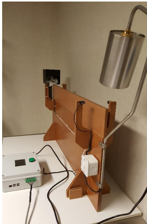
Figure 3-4: Photograph of the balance beam. Mice were placed on the light end of the balance beam and the length of time taken to cross the centre 80 cm of the beam was measured as the mice made their way to the dark box containing nesting material at the other end.
