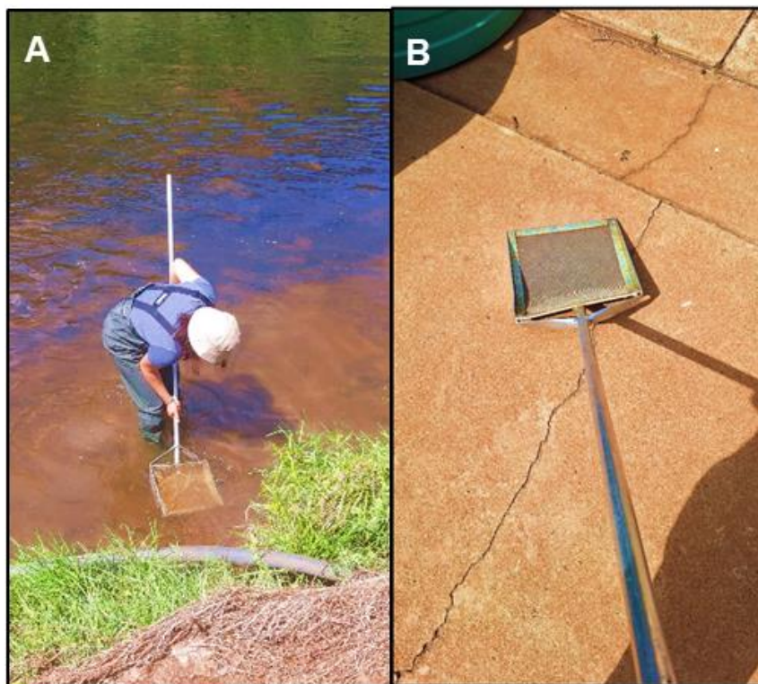
Figure 3.1 (A) Bivalves being collected using a snail sampler, (B) a metal frame snail sampler.
