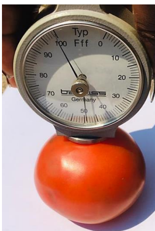
Figure 4.8: A Bareiss HP-Fff mechanical fruit firmness tester. Photo credit: Retang Kgaphola, 2019.
