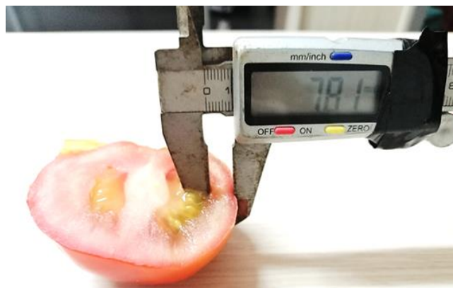
Figure 4.10: Determining pericarp thickness using a Vernier calliper. Photo credit: Retang Kgaphola, 2020.
