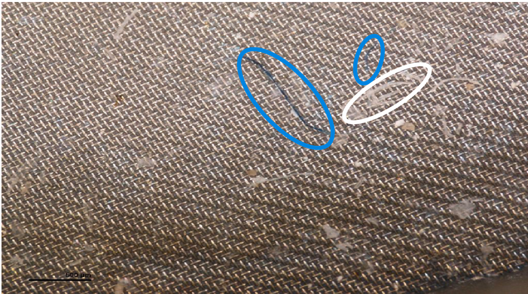
Fig. 6. Photograph of blue (blue ovals) and white (white oval) fibres on 25 µm sieve, from digested squid mantle. (For interpretation of the references to colour in this figure legend, the reader is referred to the web version of this article.)
