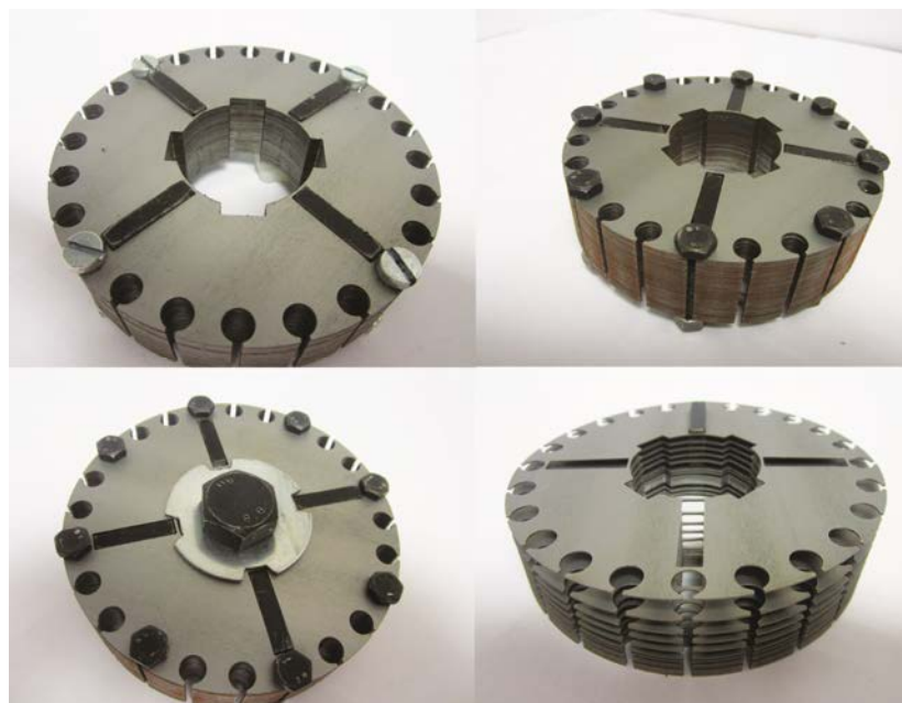
Figure 5.19: Image of quarter rotor stack assembly guide
