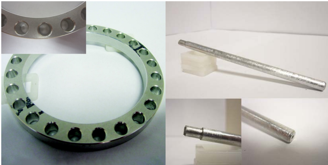
Figure 5.16: Images of rotor end rings and cage bars
