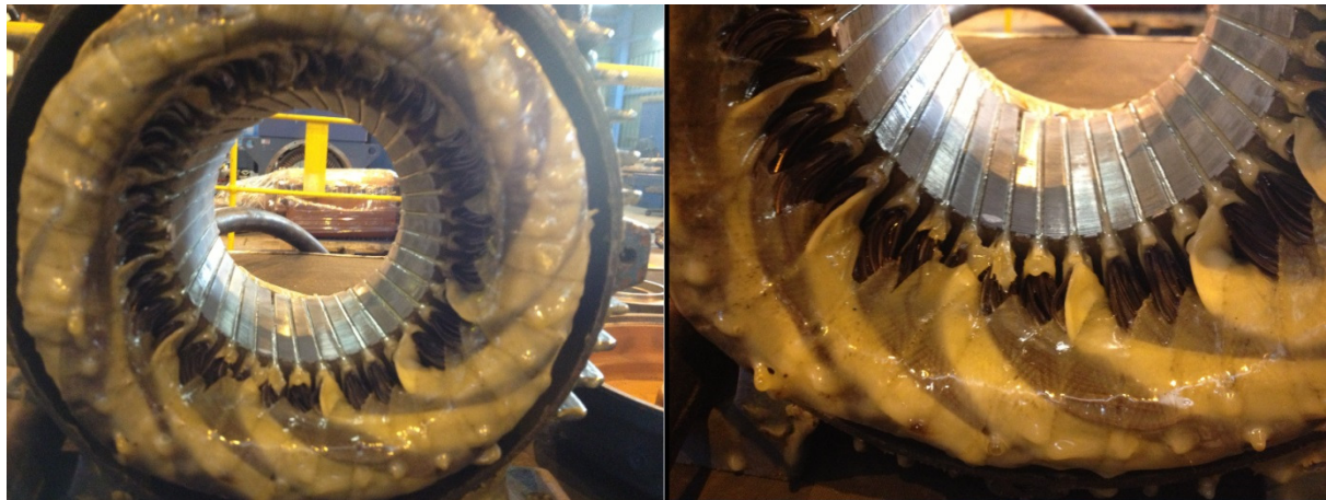
Figure 5.8: Winded stator stack after VPI
