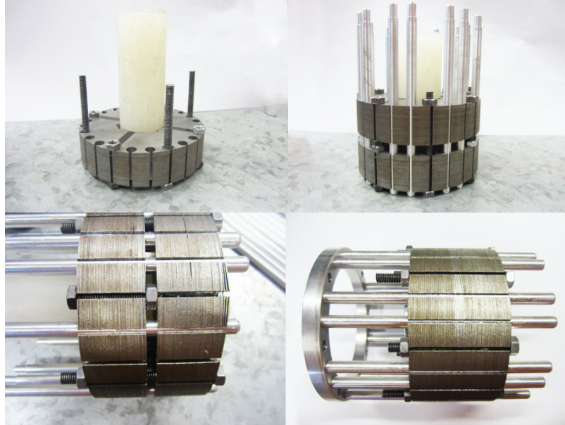
Figure 5.23: Photos of rotor assembly
