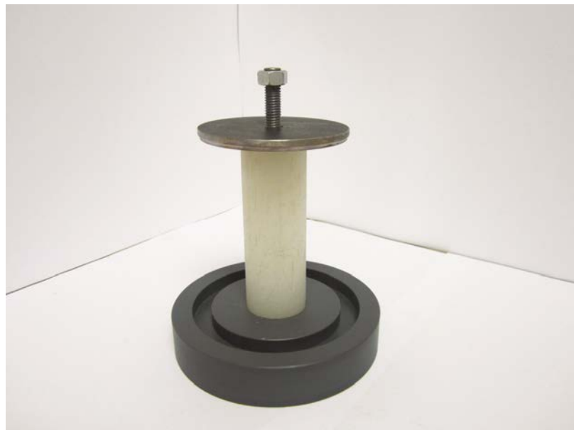
Figure 5.20: Image of rotor stack assembly jig
