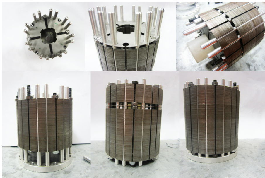
Figure 5.24: Photos of rotor assembly
