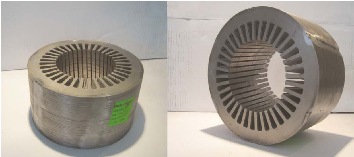
Figure 5.5: Photo of stator stack
