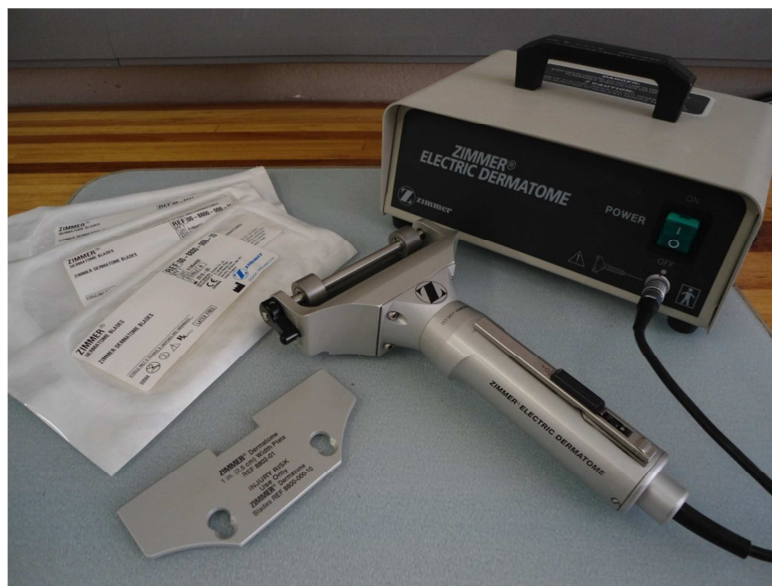
Figure E.1: Zimmer™ electric dermatome model 8821 with sterile blades and 2.5 cm width plate
