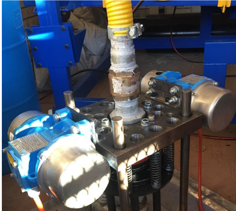
Figure 3-11: Bellow system rigid body mass and discharge one-way valve
