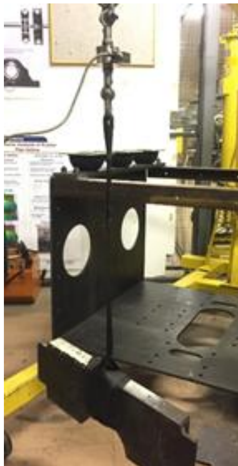
Figure 6-14: Calibration of load cell at 21.50 kg
