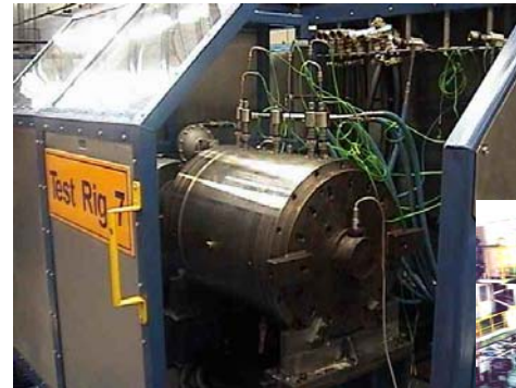
T/G Dry Gas Seal
