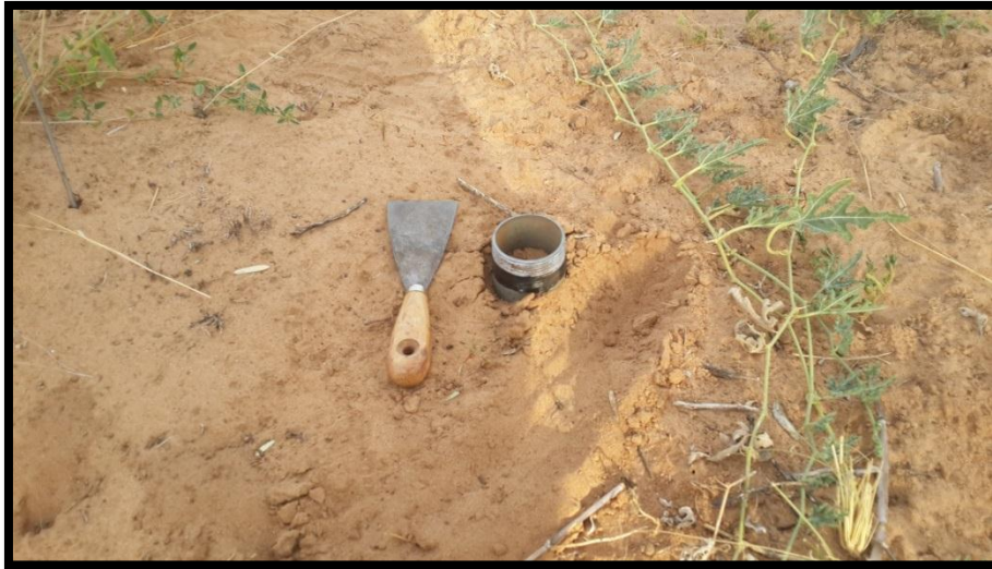
Figure 4.1: Pipe coupler and scraper used for soil sampling. Tape was used around the pipe coupler to ensure that the correct amount of soil was collected at a depth of 5 cm.
