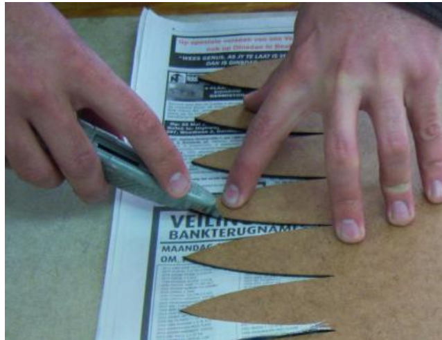
Figure 22: Illustration of MLVSI cutting using a jig over-lay on the insulation with a newspaper page as intermediate layer
