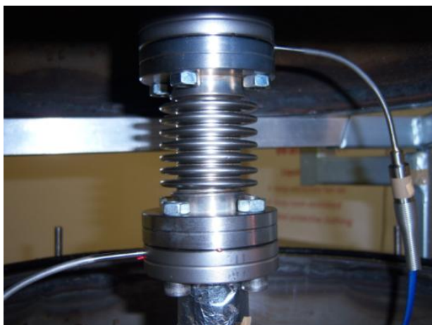
Figure 35: Photo of the coupling installed with top and bottom thermocouples shown
