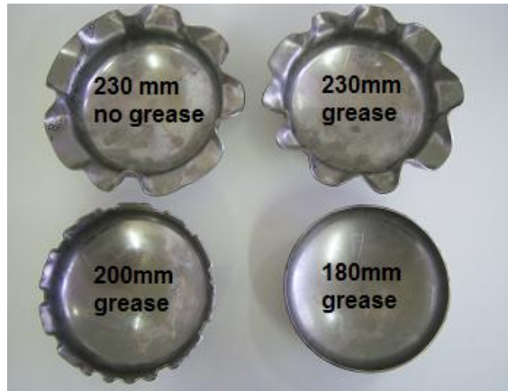
Figure 19: Manufactured 150mm Ø domes from various billet sizes
