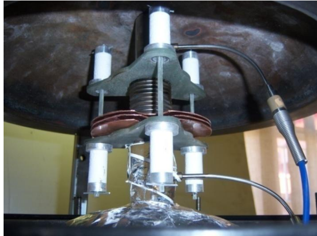
Figure 55: Photo of the manufactured and assembled optimised coupling (Coupling D)
