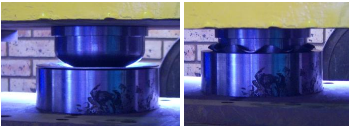
Figure 16: Inner tank dome pressing process
