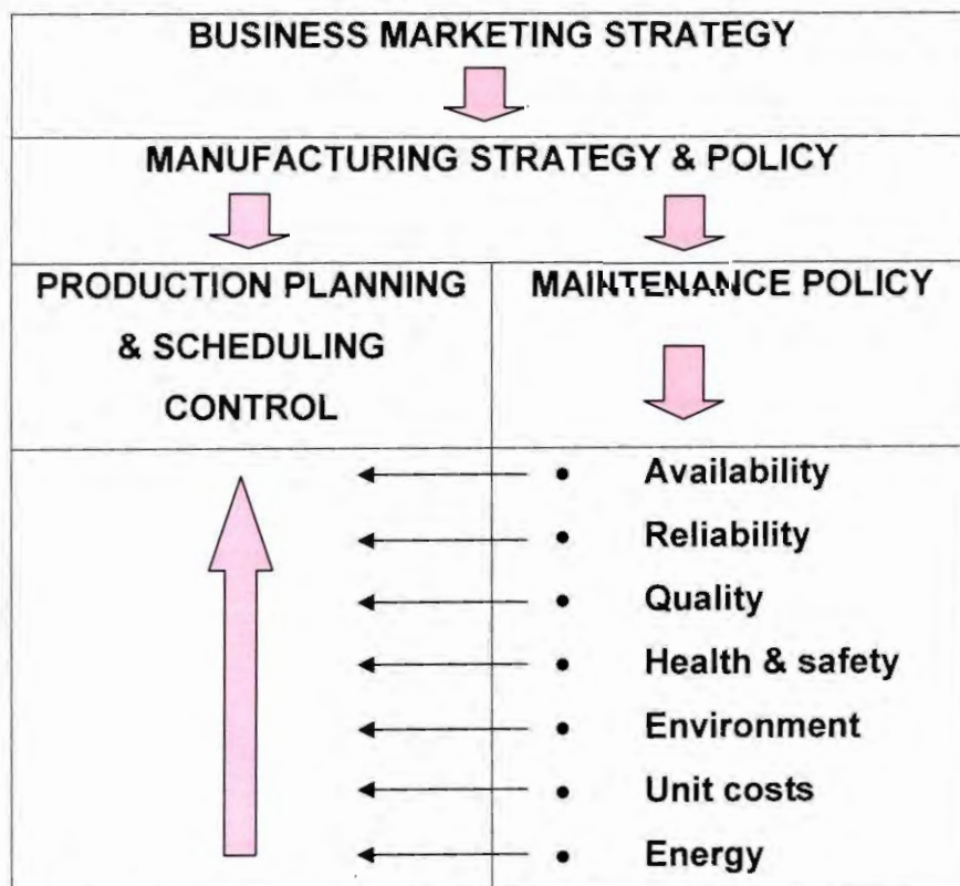
Figure 2.8: Integrating maintenance with production
