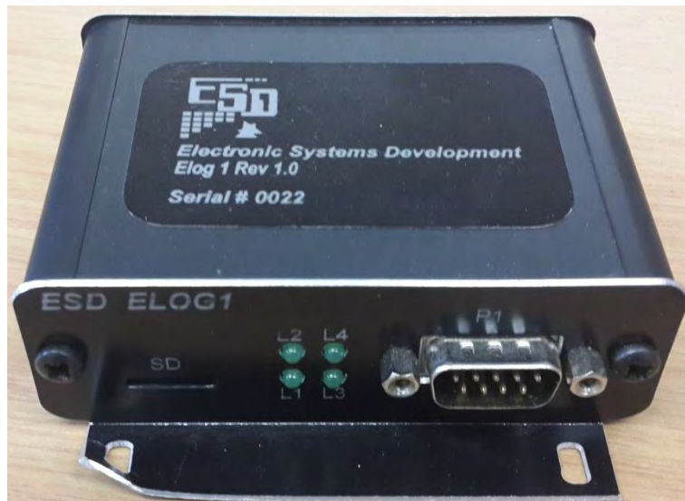
Figure 2-13: The data logger used to store data measured by the rain gauge.
