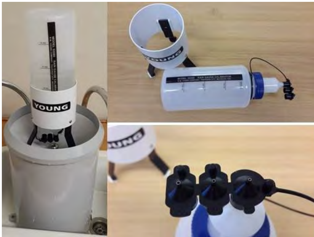
Figure 2-12: The RM Young calibrator used to ensure that the instruments are calibrated and accurate data is measured.
