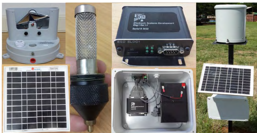
Figure 2-14: The NWU tipping-bucket rain gauge.
