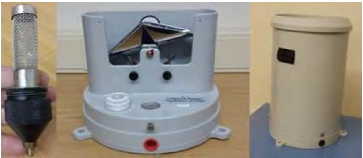
Figure 2-11: The TB3 Siphon tipping-bucket rain gauges used in the Mooi River Rain Gauge Network.
