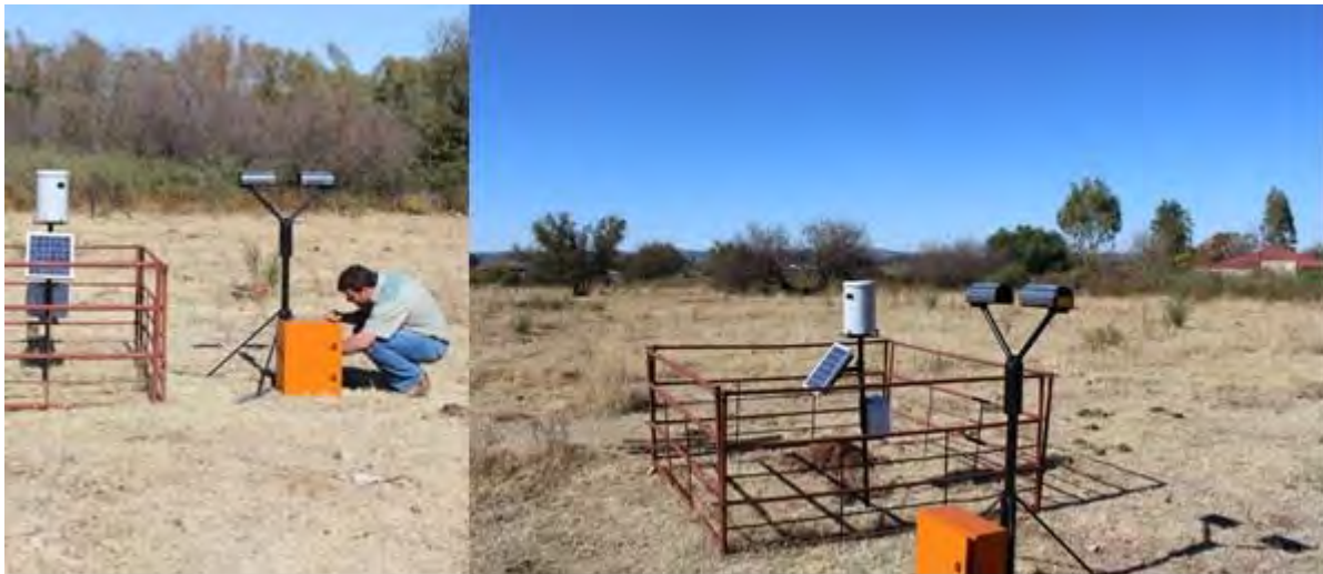
Figure 2-6: The Parsivel disdrometer deployed outside Potchefstroom, North West in close proximity to a tipping-bucket rain gauge.
