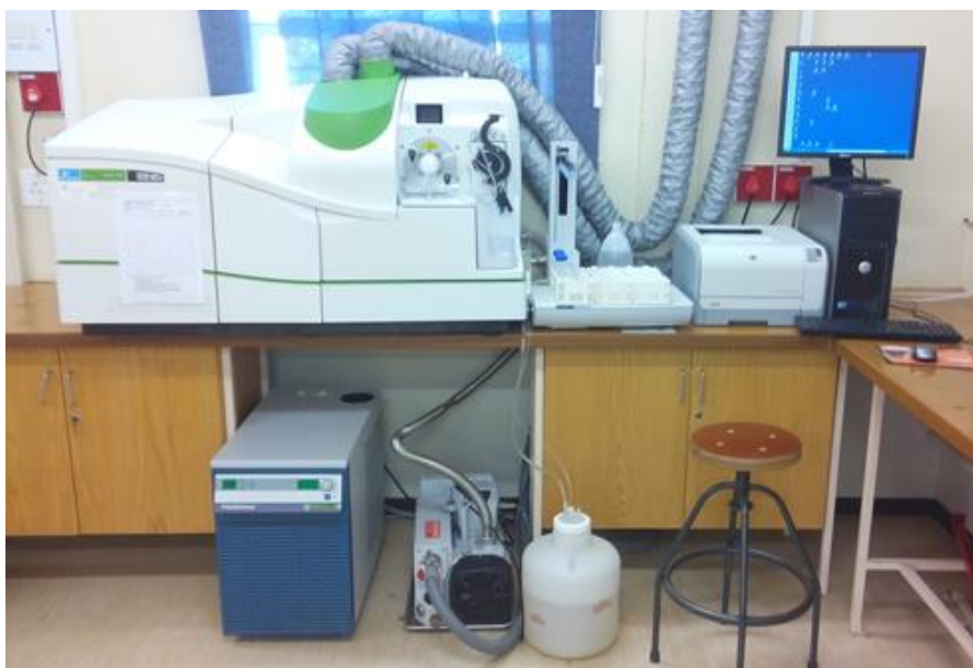
Figure H.3: The NexION 300Q Model ICP-MS system setup
