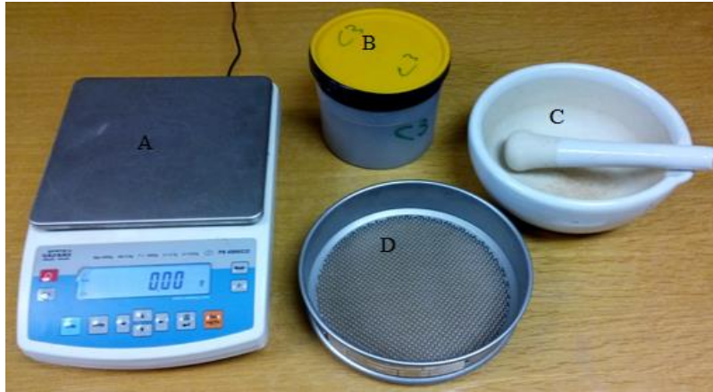
Figure 3.9: The apparatus for sample preparation: (A) a weighing scale, (B) a sealed sample inside a Marinelli beaker, (C) a mortar and pestle for crushing and homogenising samples and (D) a sieve of 2 mm mesh size.
