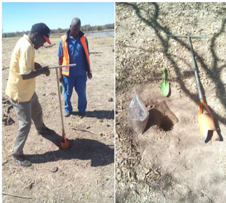
Figure 3.5: Illustration of the use of a hand auger tool for soil sampling
