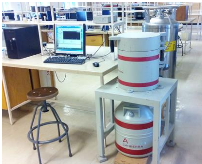
Figure H.1: Physical layout of the HPGe system
