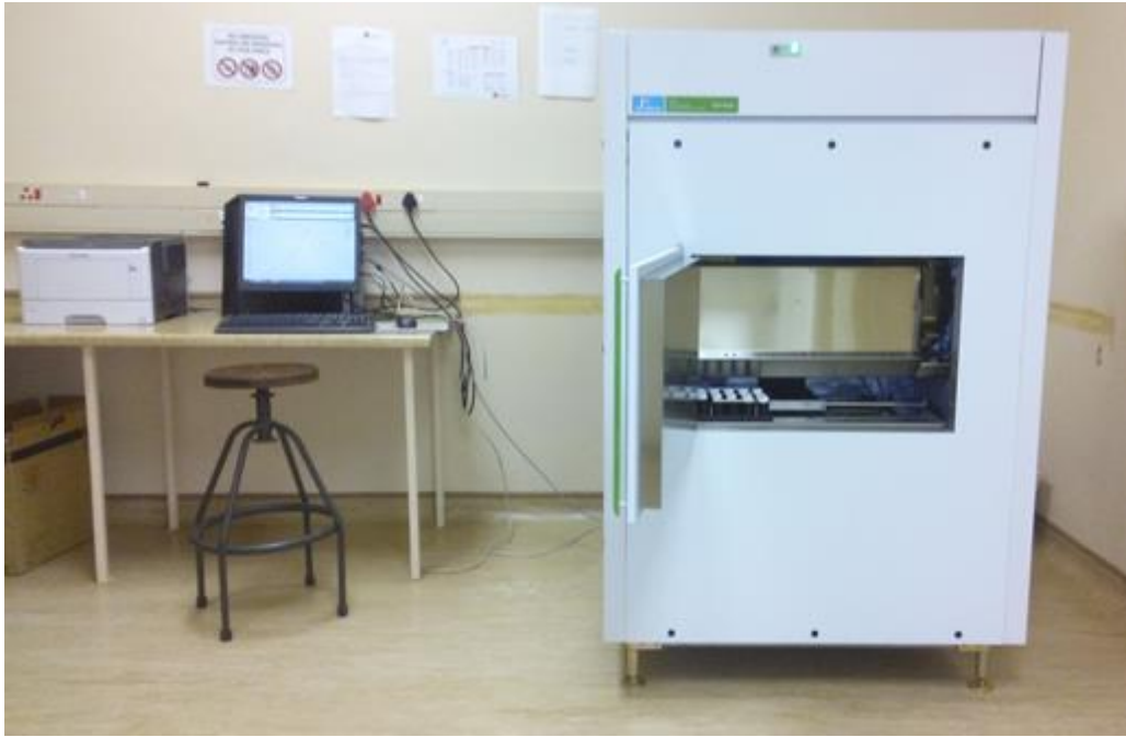
Figure H.2: The Wallac Quantulus 1220™ (PerkinElmer Life and Analytical Sciences) frontal view with open lid, showing the auto sampler trays
