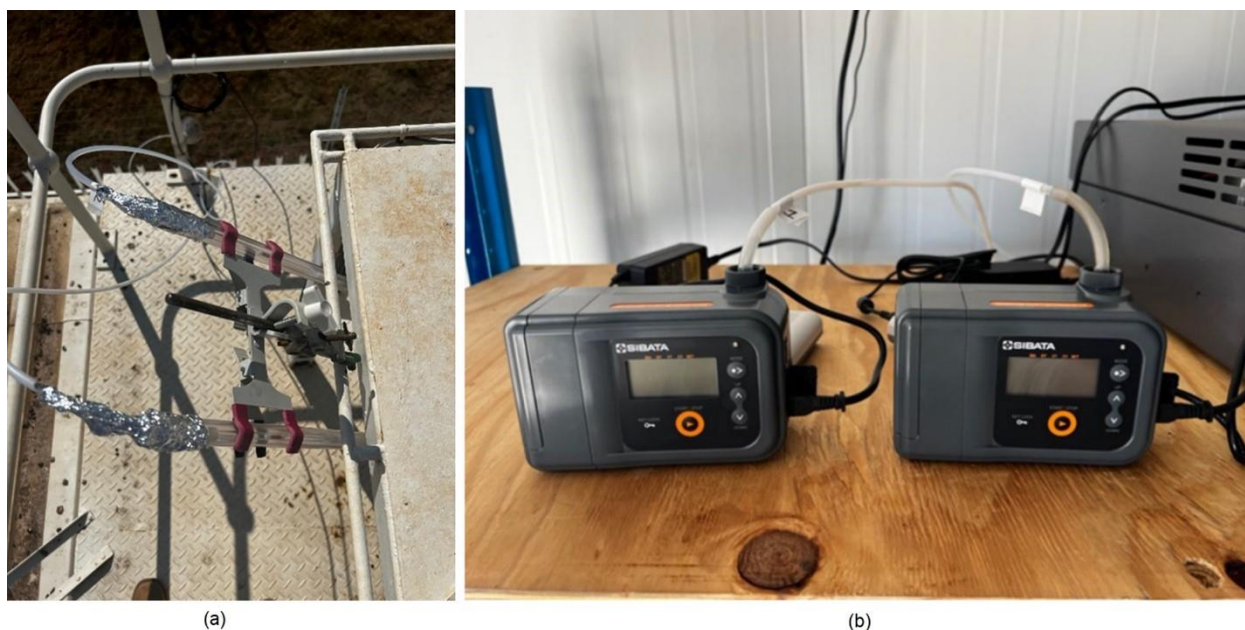
Figure 3-7: Deployment setup of the manual active sampler at Welgegund showing the simultaneous duplicate sampling of (a) gold cartridges and (b) air pumps.
