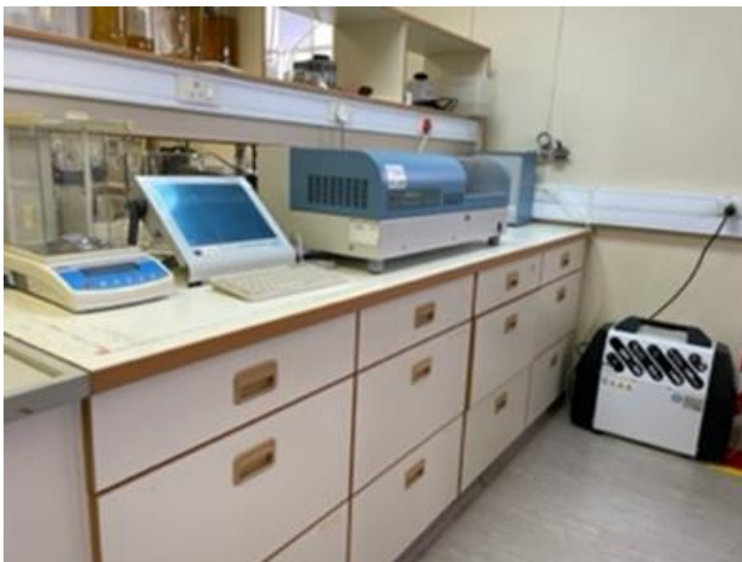
Figure 3-5: Direct Mercury Analyzer (DMA-80) system setup in a laboratory.
