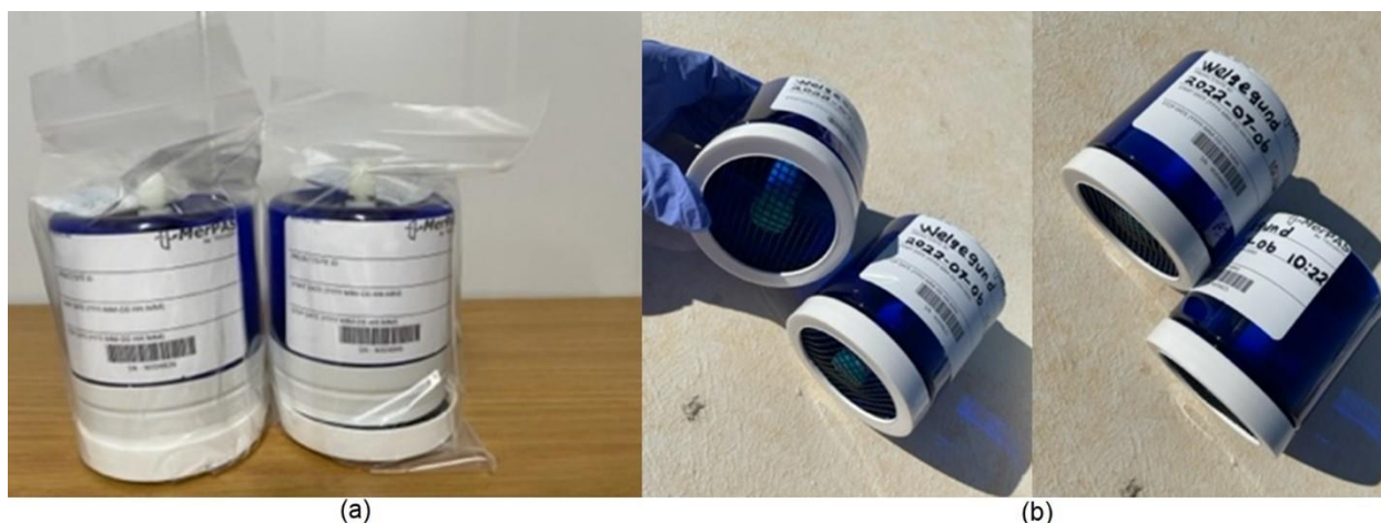
Figure 3-3: Photos of the MerPAS ® (a) samplers placed into zip-lock plastic bags, and (b) assembled samplers with black mesh screens.
