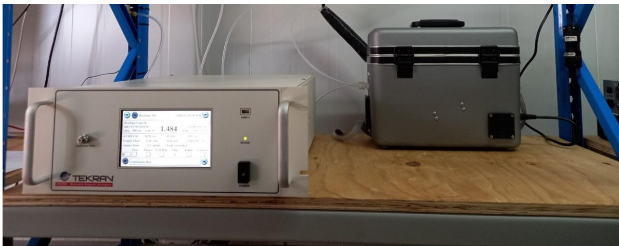
Figure 3-6: Deployment setup of the Tekran 2537X active sampler at Welgegund.
