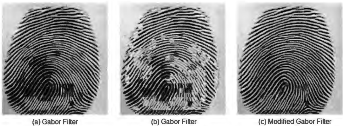
Figure 2.8: Fingerprint Images Enhancement Result for the TGF and the MGF [17]
