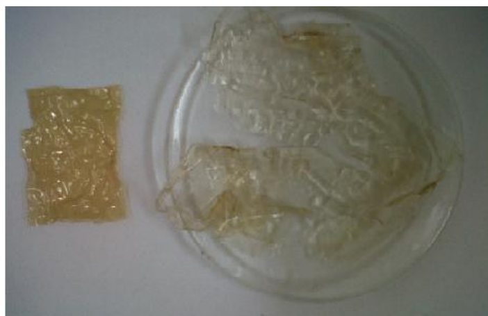
Figure 4.7: sFS-PBI blend membrane before (left) and after (right) treatment in 90wt% H 2 SO 4 .
