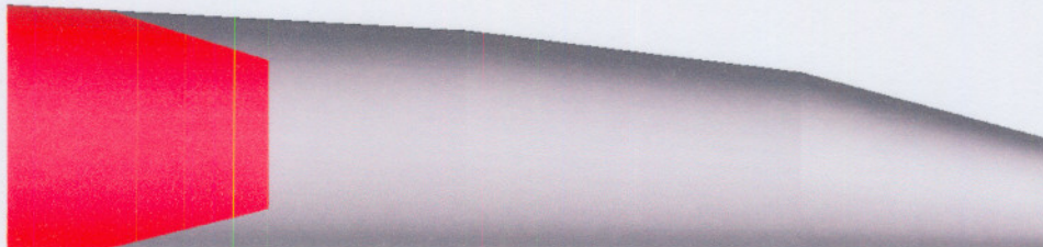
Figure 5.7: Tapering of UD carbon fabric
