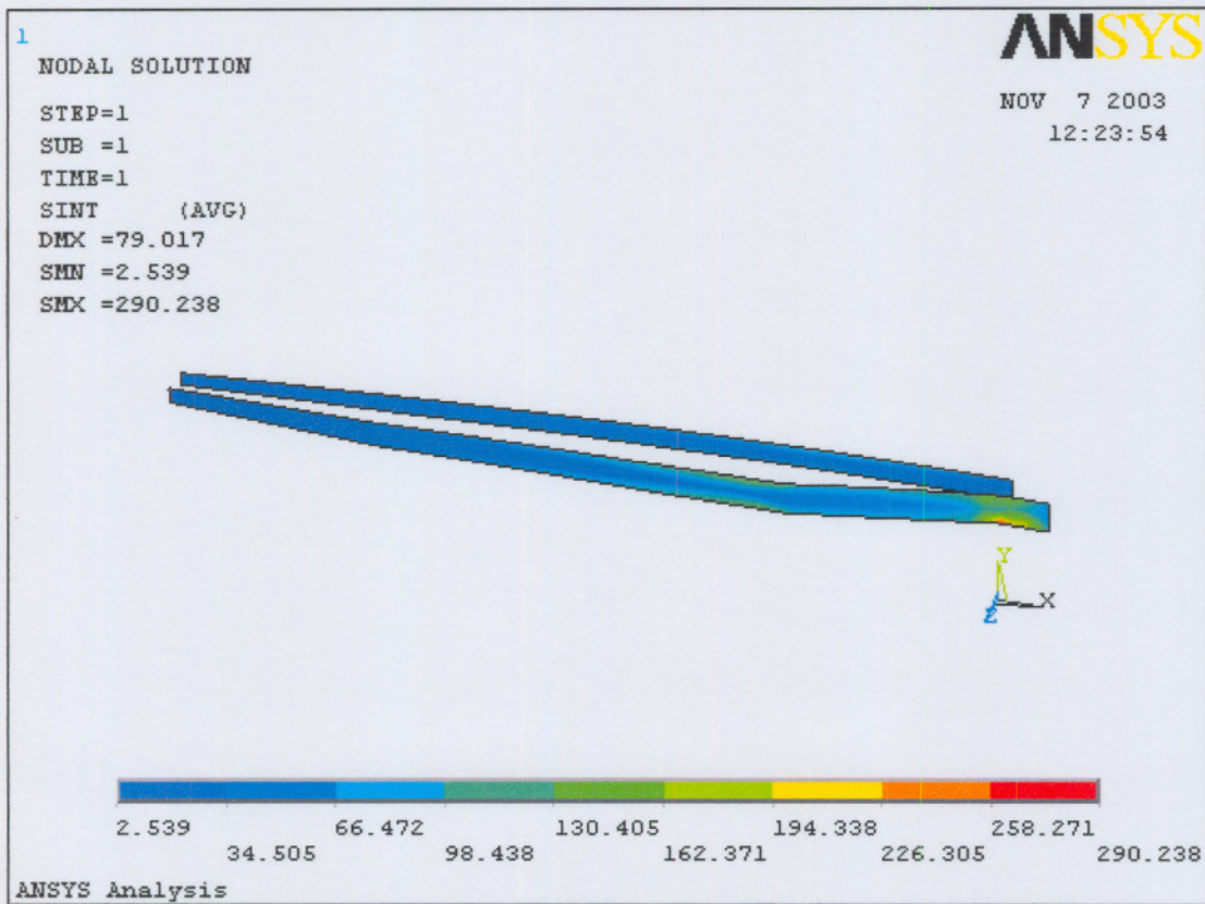
Stress Intensities - Shear Web Layer 1
