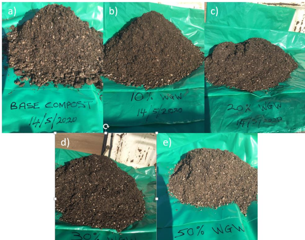
Figure 2-9: Samples collected and analysed (less than 8mm in size) after sieving of the different stockpiles. (a) Base compost, (b) 10 Gypsum wallboard waste, (c) 20% Gypsum wallboard waste, (d) 30% Gypsum wallboard waste and (e) 50% Gypsum wallboard waste.
