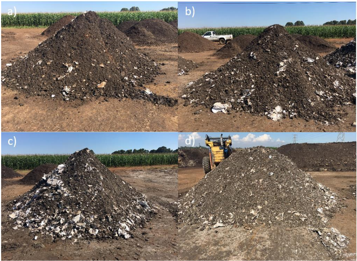
Figure 2-5: Wallboard waste and organic matter compost heaps after mixing. (a) 10% wallboard waste and 90% organic matter, (b) 20% wallboard waste and 80% organic matter, (c) 30% wallboard waste and 70% organic matter and (d) 50% wallboard waste and 50% organic matter.
