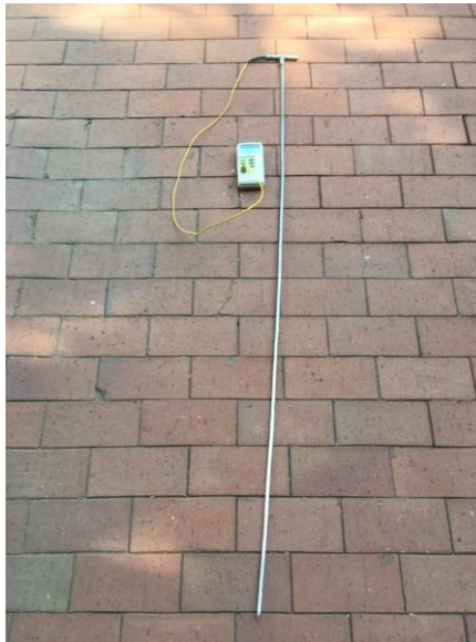
Figure 2-6: Temperature probe used to measure temperatures of the compost heaps.
