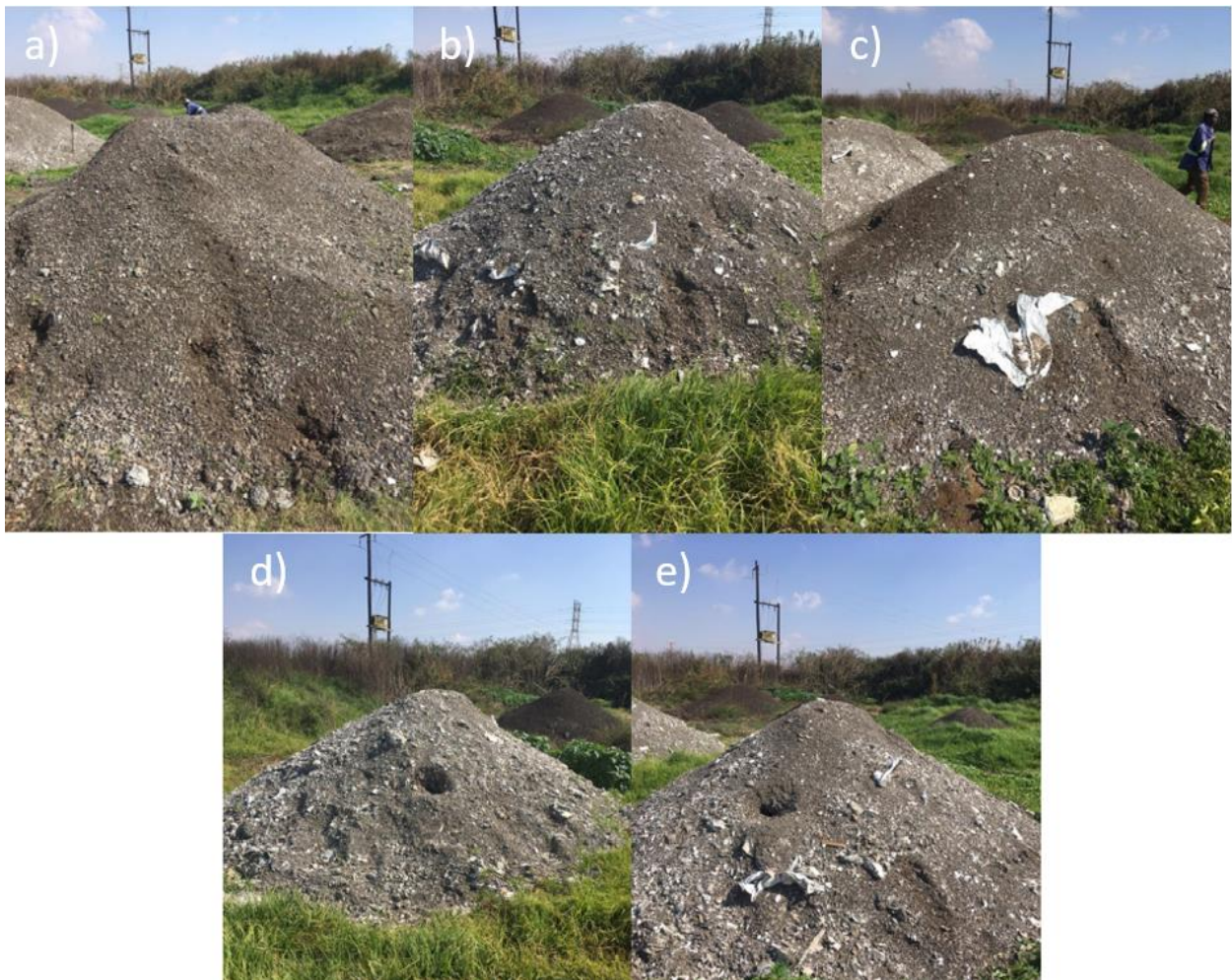
Figure 2-8: Gypsum wallboard waste and organic matter compost heaps after the completion of the trial. Control compost heap (a). 10% wallboard waste and 90% organic matter (b). 20% wallboard waste and 80% organic matter (c). 30% wallboard waste and 70% organic matter (d). 50% wallboard waste and 50% organic matter (e).
