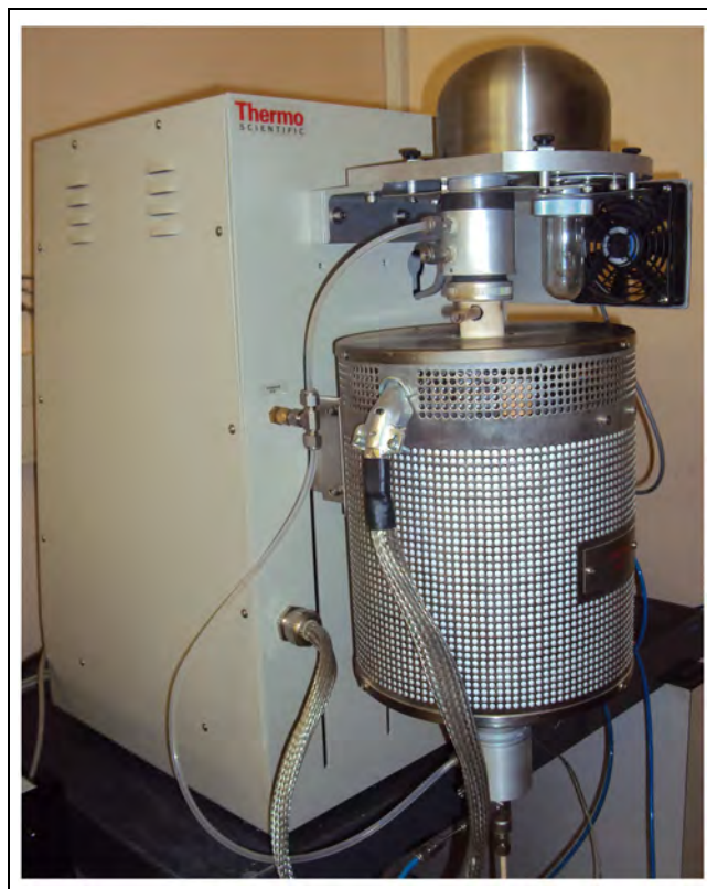
(a) A photograph of the ThermoMax700 TGA
