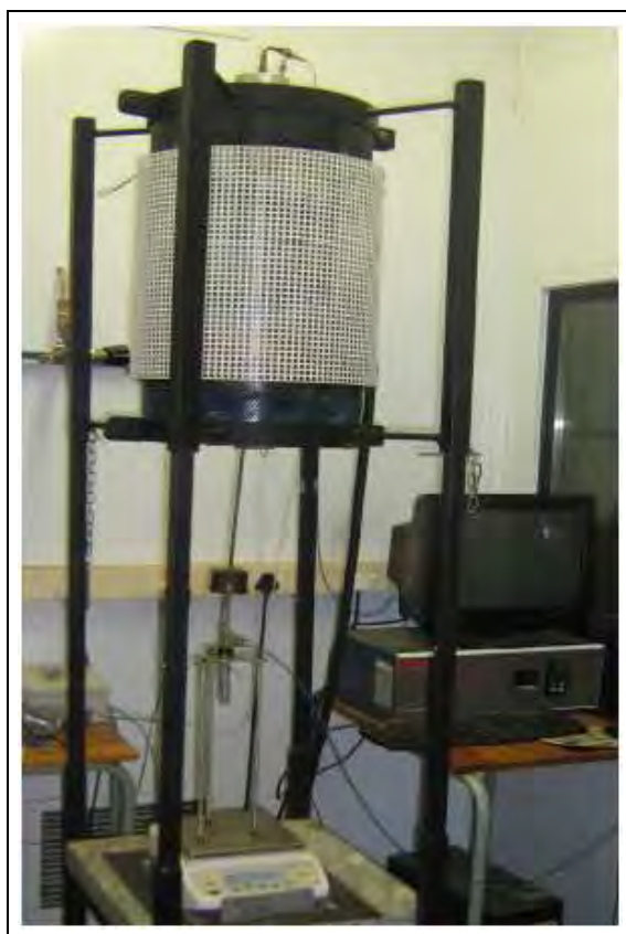
(a) A photograph of a packed bed reactor
