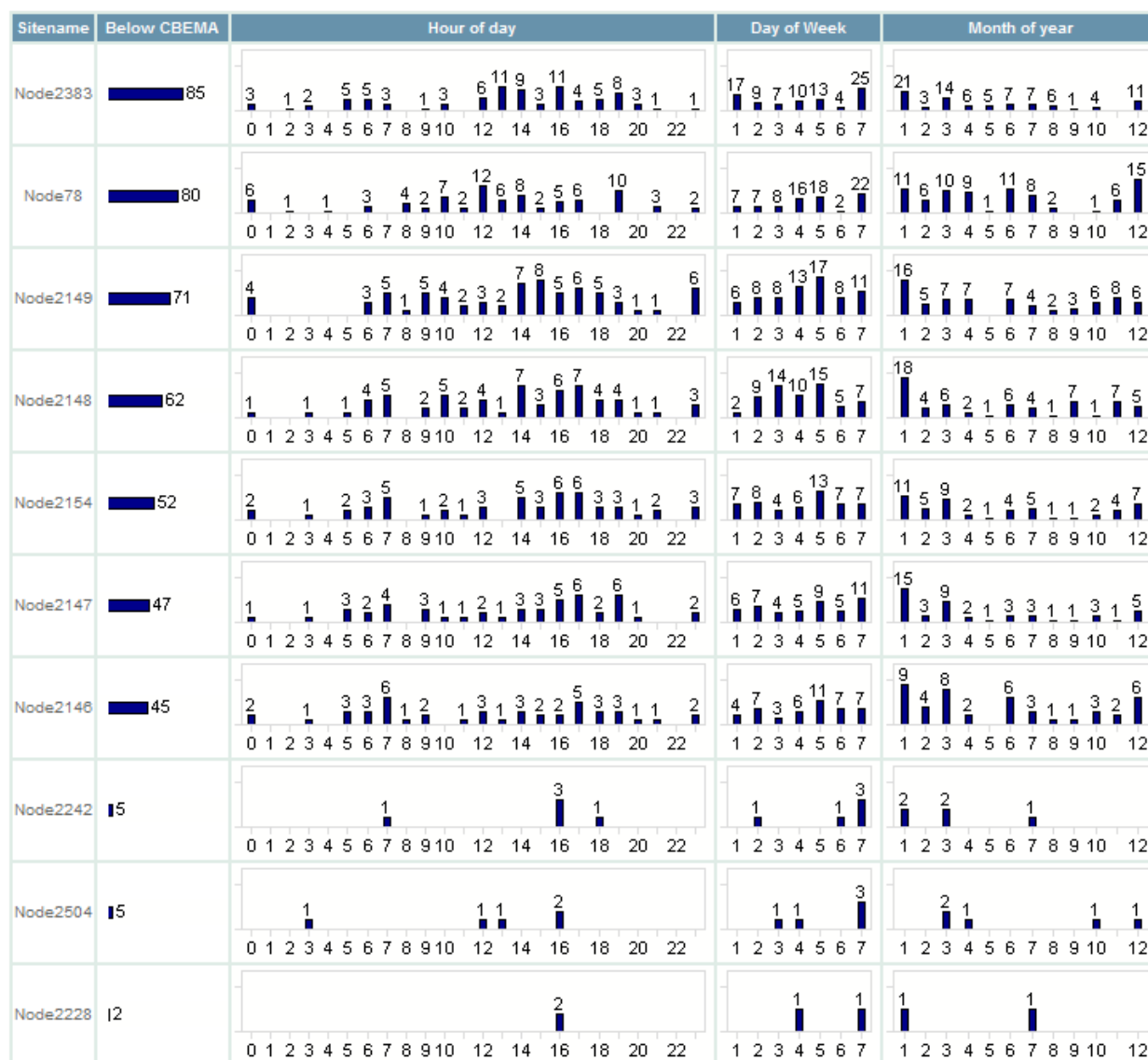
Figure 4-17 Time distribution of dips below the CBEMA curve for several sites of a utility over a period of 4 years
