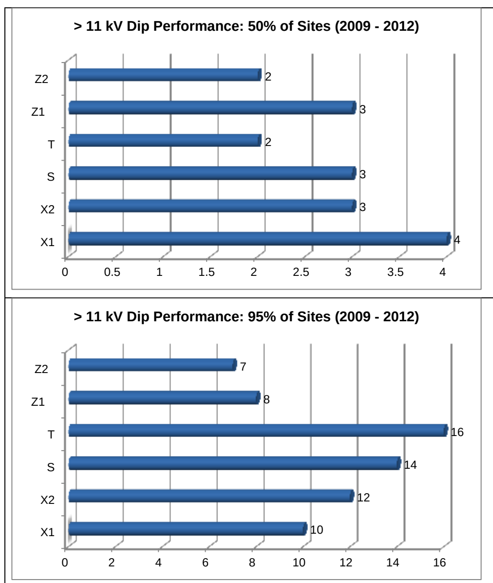
Figure 4-9: Comparison of characteristic dip numbers for networks = 11 kV
