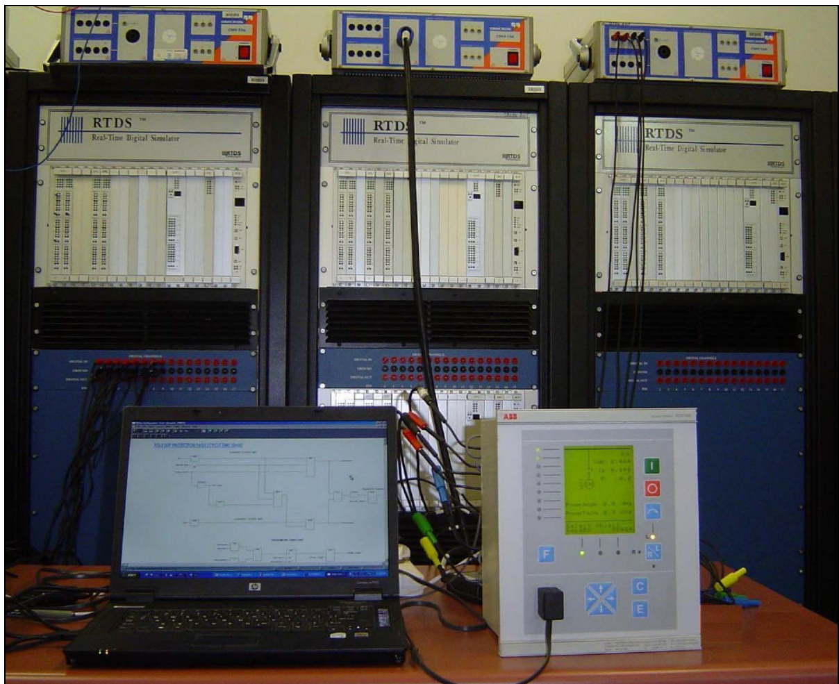
Figure 6.2: ABB REM543 relay testing with RTDS
