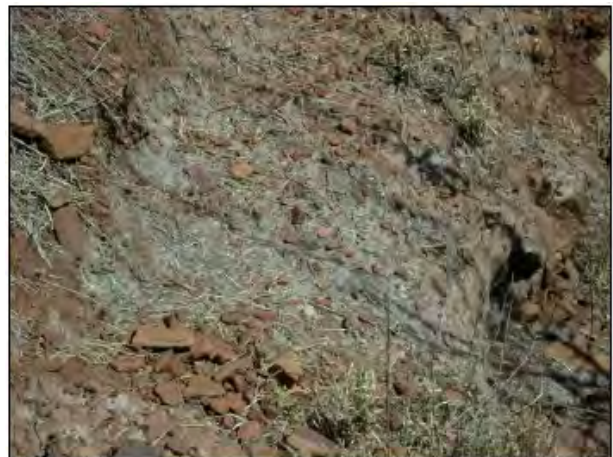
Figure 3-7: Loose asbestos fibres at Zeelig dump indicating secondary pollution on the dump after rehabilitation.
